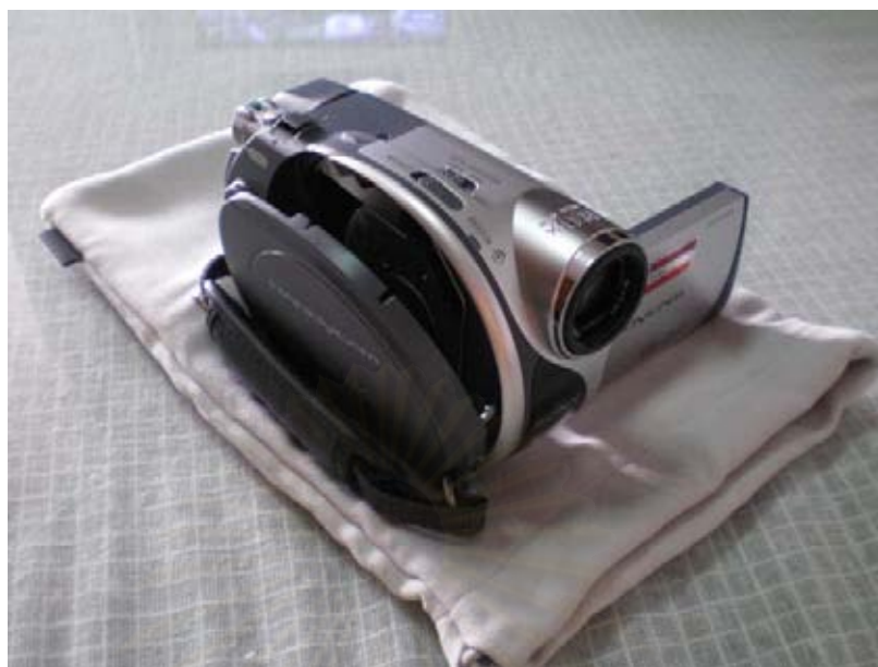
Figure 3.1. Video recorder with mini-DVD recording system (SONY, DCR-DVD605E).
