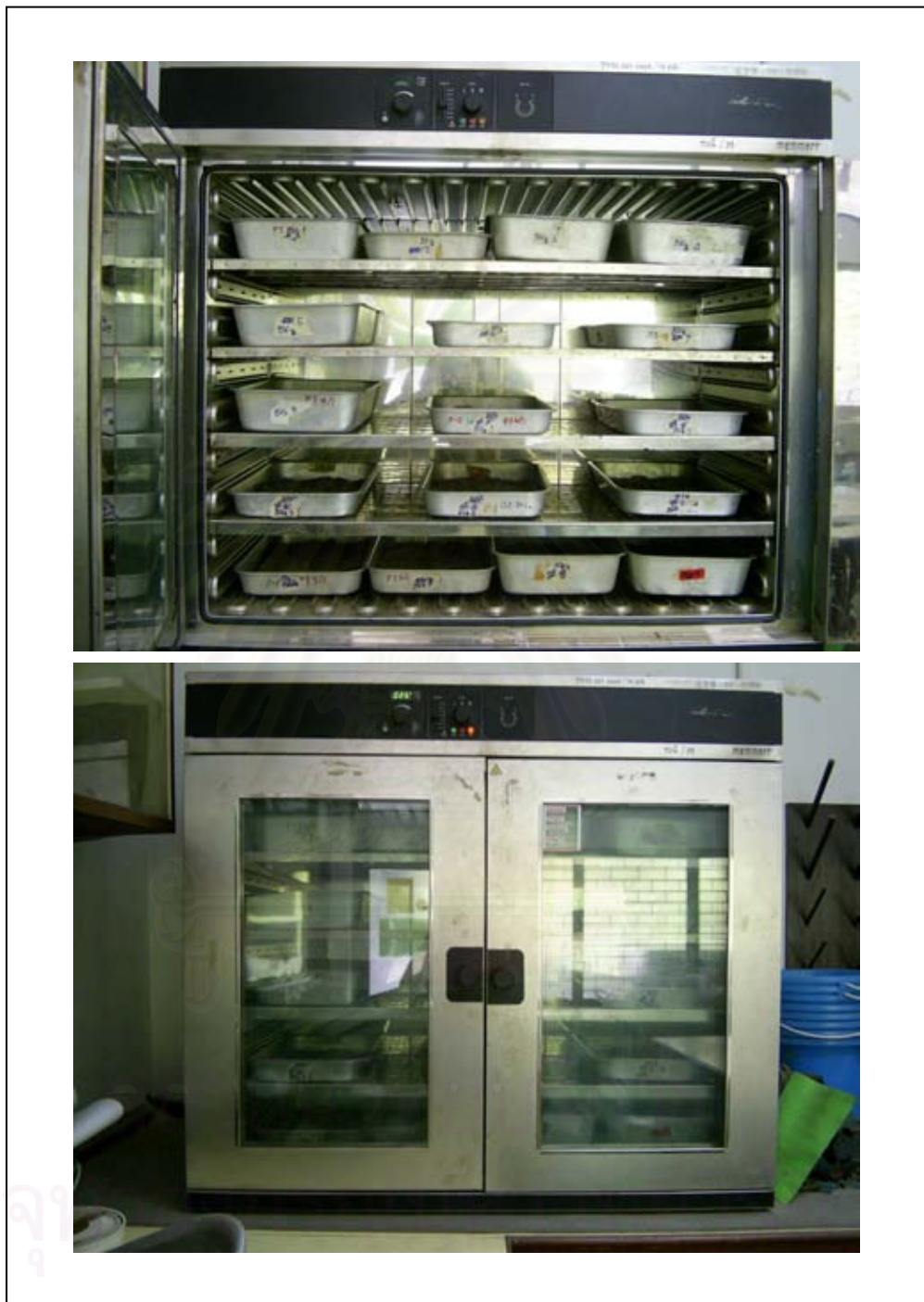
Figure 3.9 Photographs show drying samples in oven at temperature 80° C about 5-6 hours for release water in samples.
