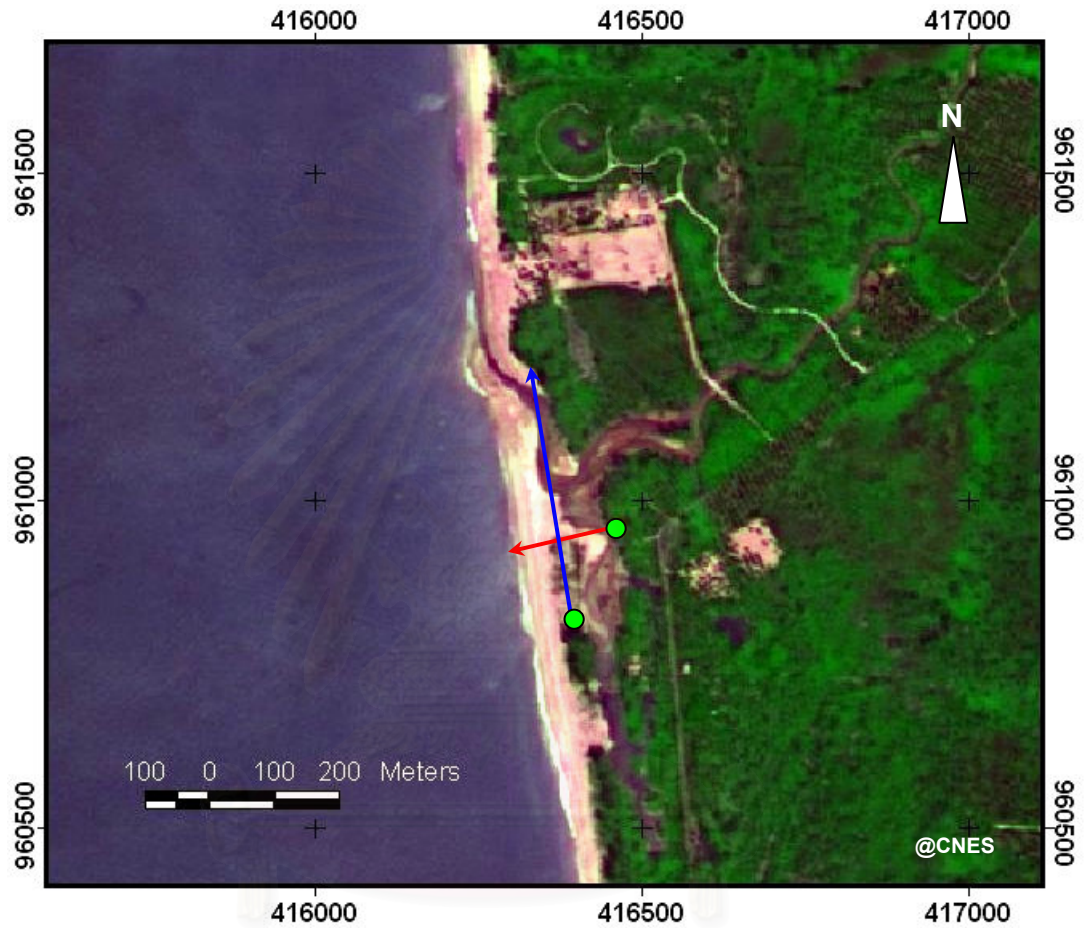
Figure 4.66 Beach profiling lines both perpendicular and parallel to the shoreline at Klong Khuek Khak. Green dot is a reference point. Red line is east-west beach profile and blue line is south-north inlet/outlet cross-section. Background image is from SPOT-5 satellite taken two year after the 2004 tsunami.
