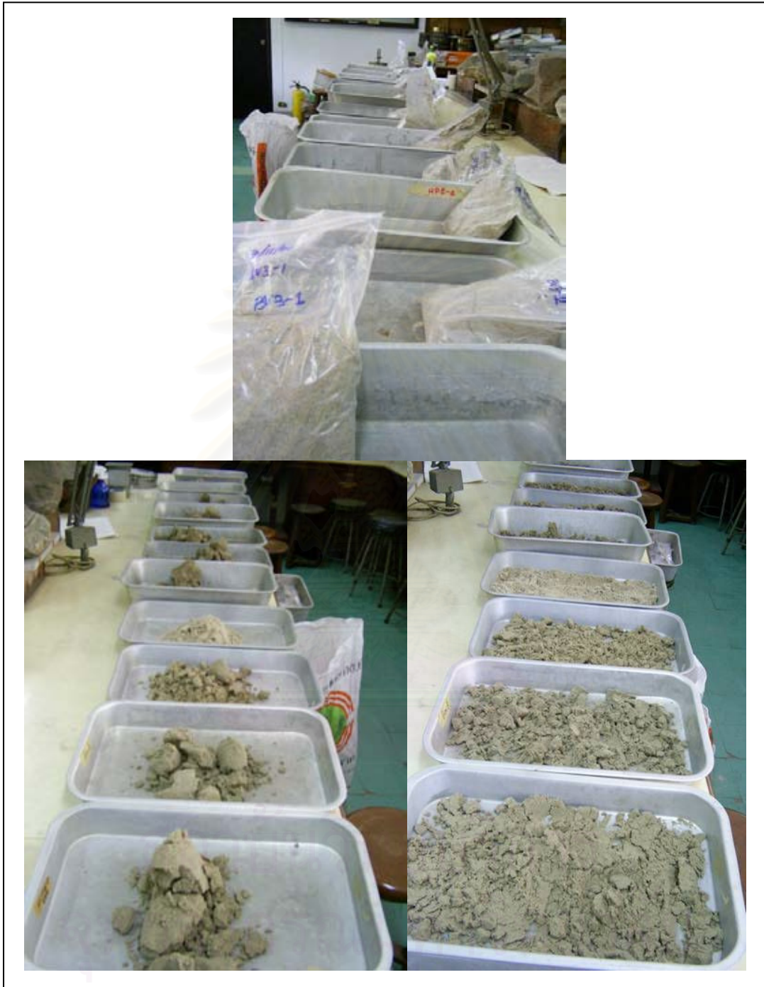
Figure 3.8 Photographs show preparing of samples before dry in oven and sieve in dry sieve mesh.
