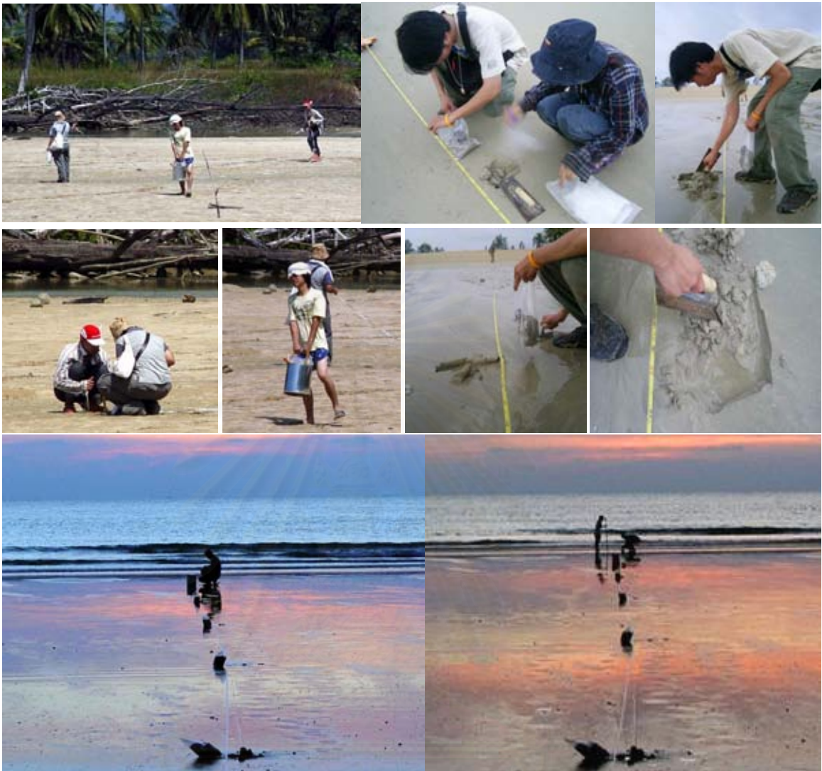
Figure 3.6 Photographs show surficial beach sediment sampling from backshore to foreshore in swash zone at low tide time.
