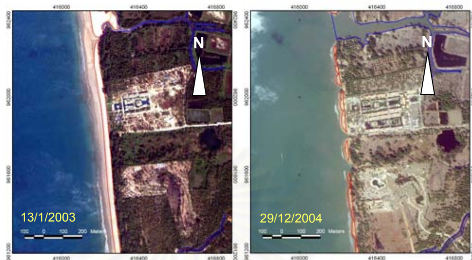
Figure 4.19 Comparing IKONOS satellite images taken before and after tsunami show eroded beach area at area C which split into several parts from the erosion of tsunami and shape of beach is change into half-circle shape similar to the cusped beach morphology. Red polygon indicated beach area in each period.
