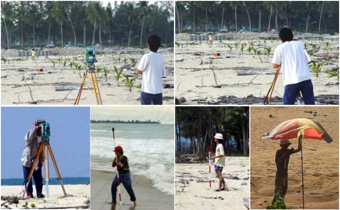
Figure 3.5 Photographs showing measurement of beach profile and inlet/outlet cross-section in the study area.
