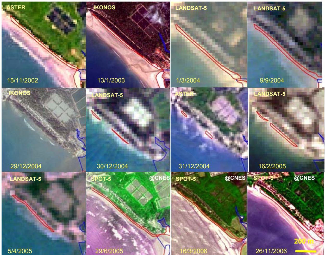
Figure 4.14 Series of satellite images showing beach area change at area A before and after the 2004 tsunami event. Red polygon in each image indicated beach area from mean high tide shoreline.
