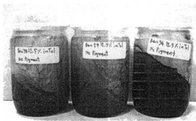
Figure 4.2 Suspension gels of three organoclays prepared by a homogenizer.
