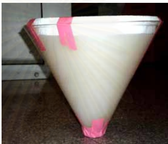
Figure 3.5 The agar cone phantom simulate pediatric patient.
