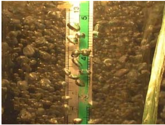
a) Superficial Gas Velocity = 0.011 m/s Top Section
