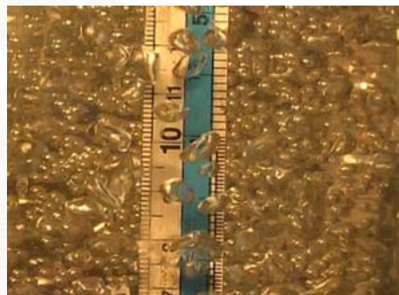
b) Superficial Gas Velocity = 0.016 m/s Middle Section
