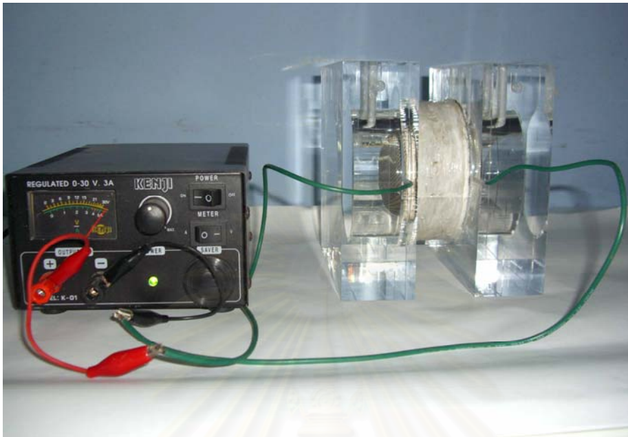
Figure A3. Power supply and chamber used in the accelerated test of chloride diffusion coefficient
