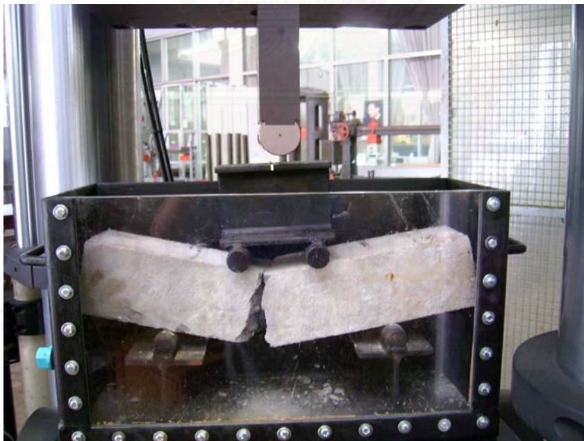
Figure A2. Fracture of concrete beam under bending load
