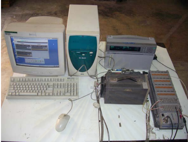
Figure A1. Equipments used to collect bending load and deflection of concrete beam under flexural cyclic load
