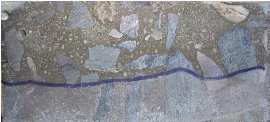
Figure A4. Chloride penetration depth of specimen M2 subjected to the accelerated test of chloride diffusion coefficient
