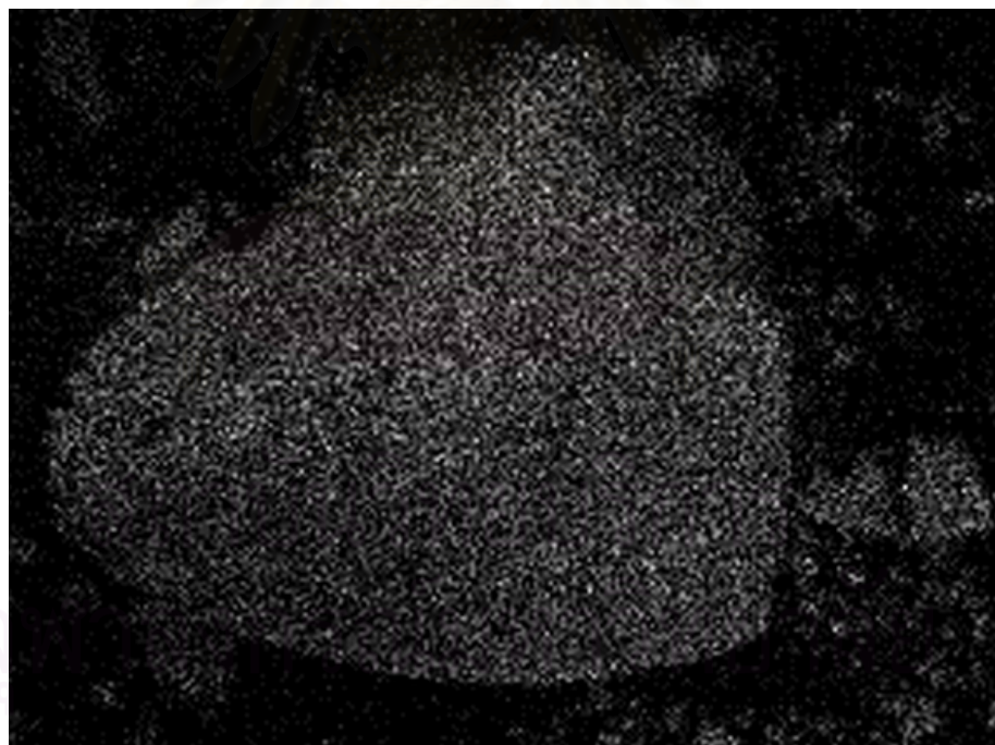
Figure 5.28 (b) SEM elemental mappings of cobalt on the exteriors of Co/S-AA
