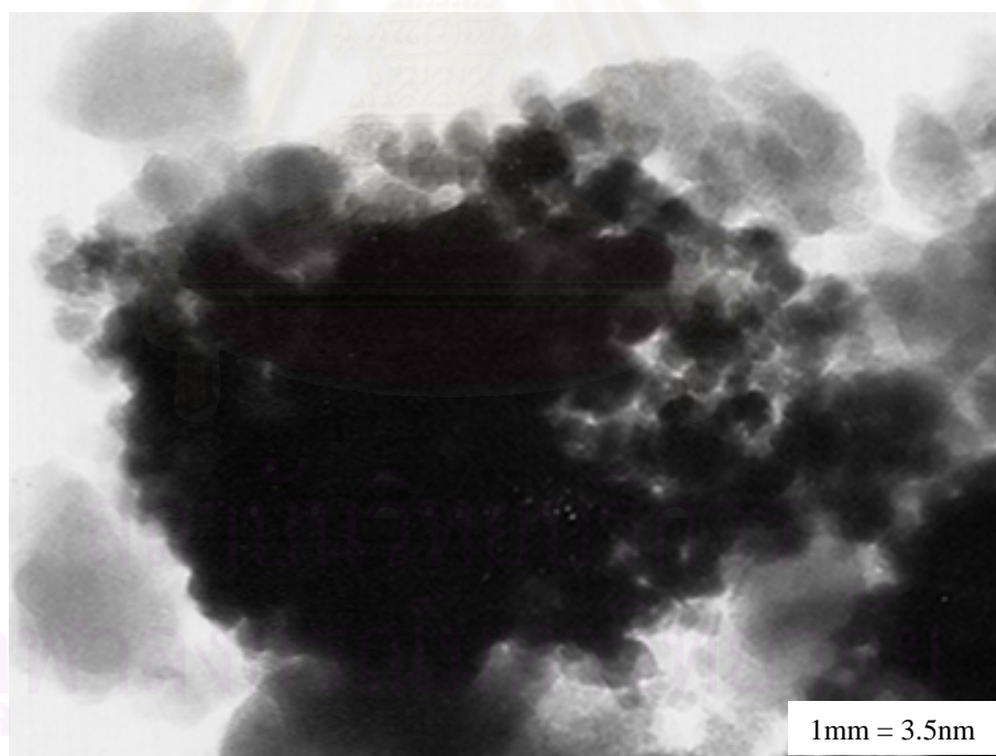
Figure 5.10 (a) TEM micrographs of Co/M-Ac.
