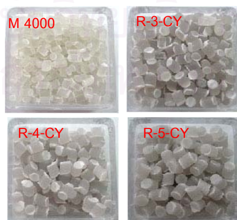
Figure 4.18 Color of masterbatches with different cristobalite powders
