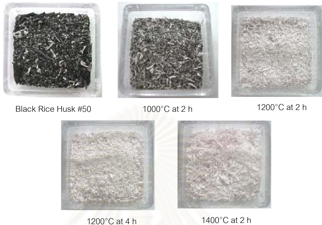
Figure 4.11 Appearance of heat treated B-RHA at various conditions, from 1000 to 1400°C for 2 h and 4 h
