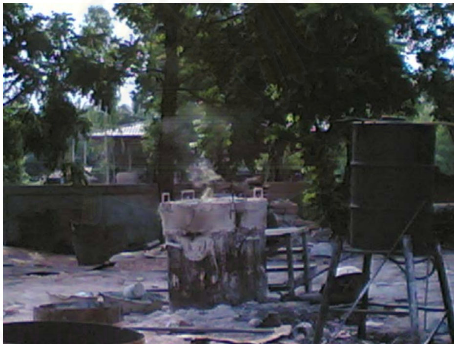
Figure 4-8 Brass furnace by used lubricant oil
