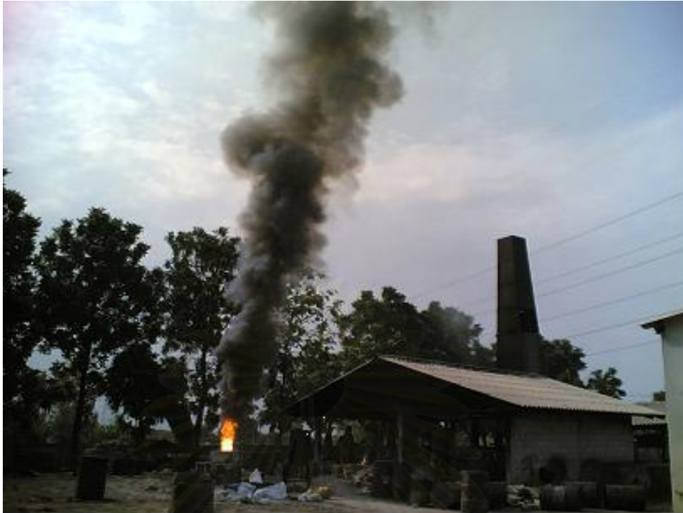
Figure 4-9 Brass melting by used lubricant oil fueled
