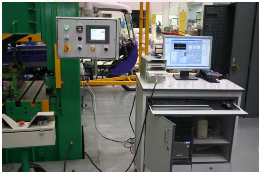
Figure 3.8 Two hundred ton of hydraulic press machine and blank holder force control system
