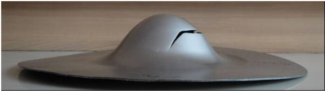
Figure 7.20 Front view of part with constant BHF of 63,125 N (full as 25.25 tons) and constant pressure of 4 MPa
