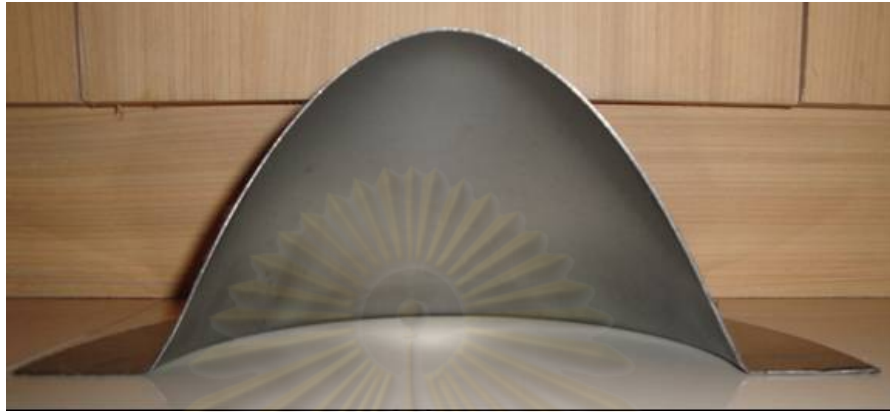
Figure7.30 Parabolic part with constant BHF of 63,125 N (full as 25.25 tons) and constant pressure of 3 MPa in half-section view
