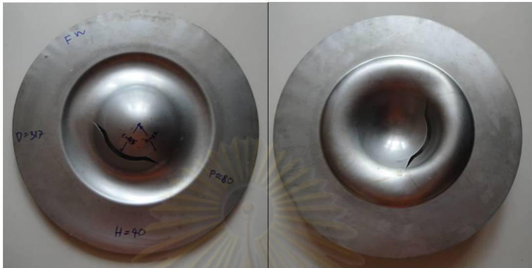
Figure 7.23 Top and bottom view of part with constant BHF of 63,125 N (full as 25.25 tons) and constant pressure of 8 MPa
