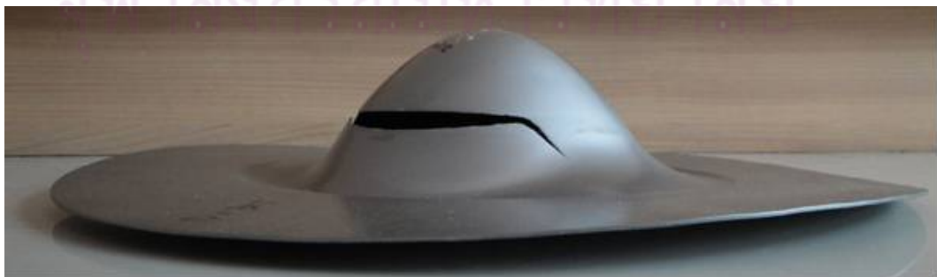
Figure 7.22 Front view of part with constant BHF of 63,125 N (full as 25.25 tons) and constant pressure of 6 MPa
