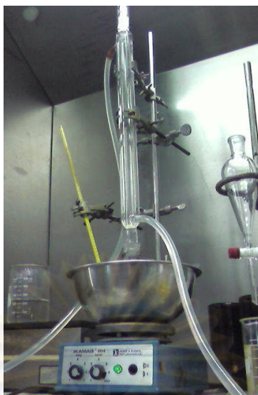
Figure 3.1 Glass reactor with heating plate and magnetic stirrer
