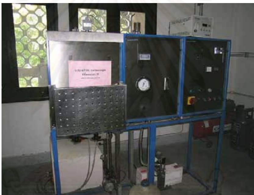
Figure 1.12 Linn electrical furnace model HT 1800 Plus VAC Bottom Loader based at the Department of Geology, Faculty of Science, Chulalongkorn University.
