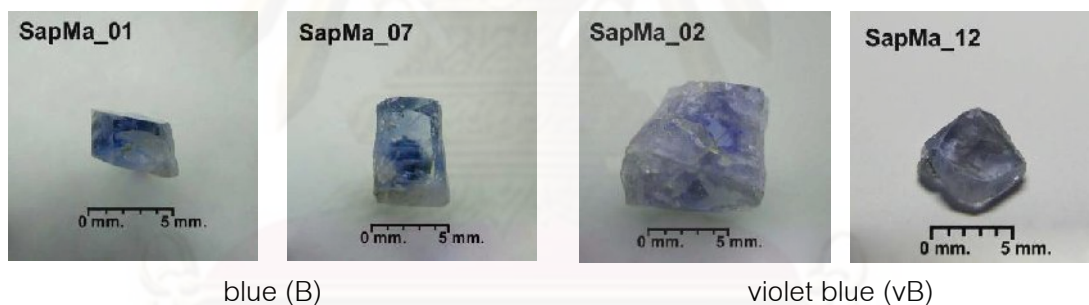
Figure 3.4 Different body colors in light blue variety of samples in which their color codes are based on the GIA Gem Set.
