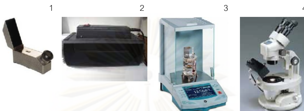
Figure 1.2 Basic gem equipments, including 1. refractometer, 2. ultraviolet lamps, 3. electronic balance and 4. gemological microscope, all based at the GIT.
