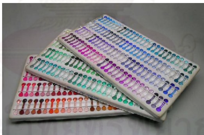
Figure 1.3 GIA Gem Set belonging to the GIT used for color coding of the sample.
