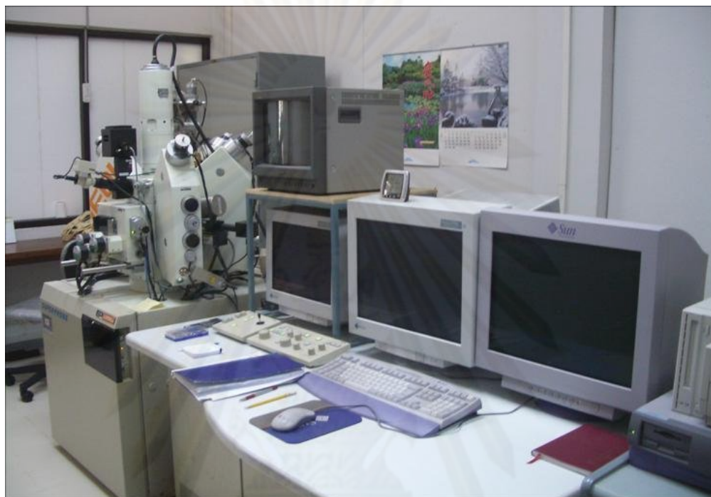
Figure 1.10 JEOL Electron Probe Micro-Analyzer (model JXA-8100) based at the Department of Geology, Faculty of Science, Chulalongkorn University.
