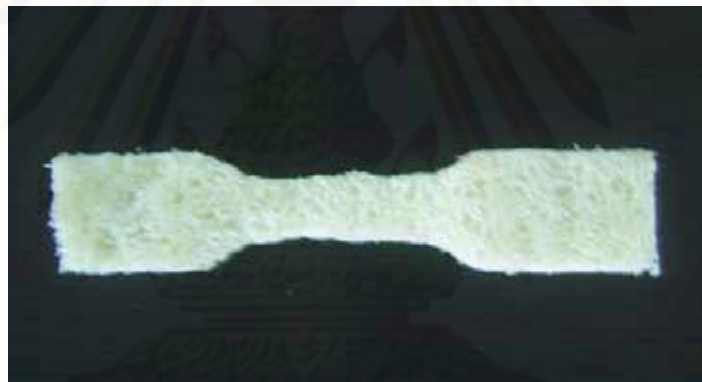
Figure 4.4 Tensile specimen of LDPE/EVA Blend Foam
