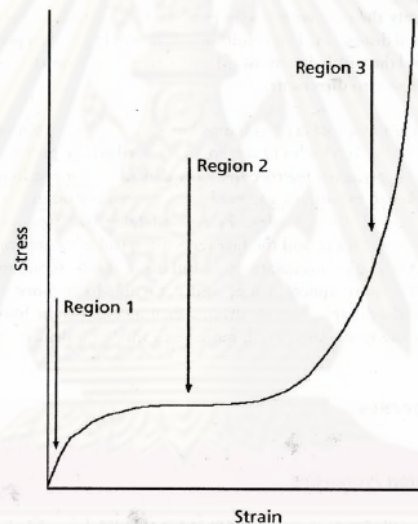
Figure 2.3 Schematic compression stress-strain curve for foam [2]
