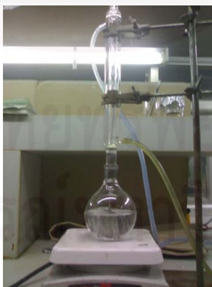
Figure 4.9 Gel content test of LDPE/EVA Blend Foam
