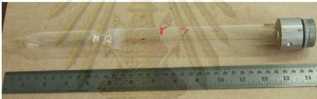
Fig. 3.5 Prepared ampoule crucible with 22 mm inside diameter
