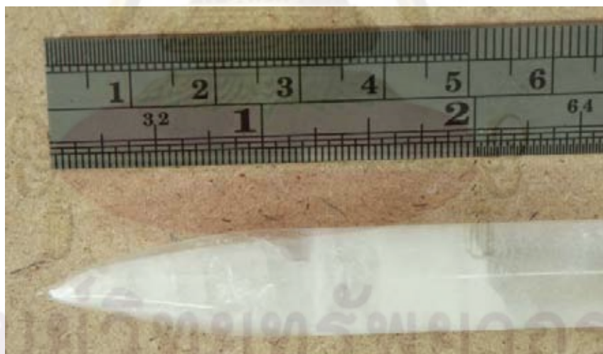
Fig. 4.9 Grown crystal of \text{LaCl}_3:\text{Ce} with clearer and partially cracked interior
