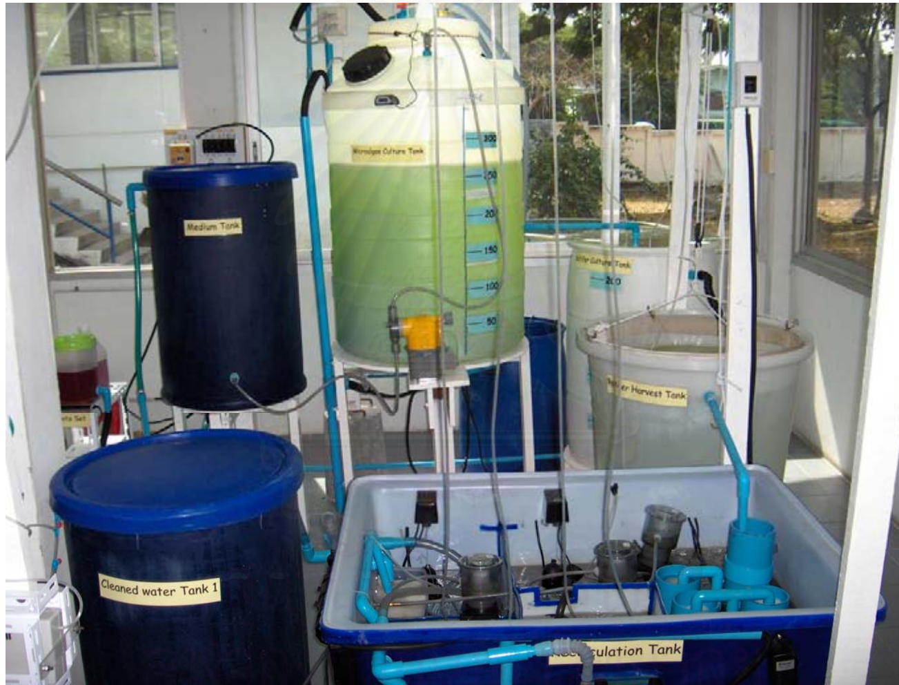
Figure 5.2 Photograph of a closed-recirculating, continuous culture system for microalga ( T. suecica ) and rotifer ( B. plicatilis ).
