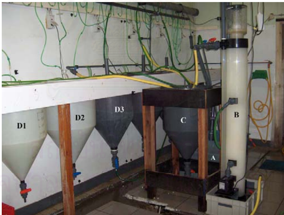
Figure 4.1 Diagram (top) and photograph (bottom) of the recirculation system. A = Settlement tank, B = Protein skimmer, C = Biofilter tank, D1-6 = Rotifer culture tanks, E = Food storage, PP = Peristaltic pump, → Direction of flow.
