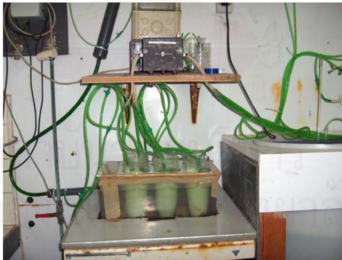
Figure 4.3 Refrigerated feed suspension distributed to the individual rotifer tanks by mean of a peristaltic pump.
