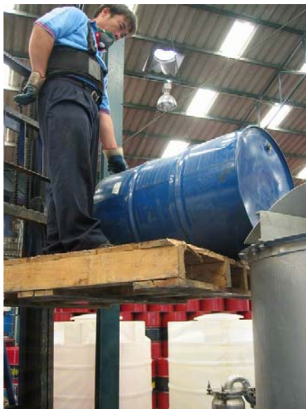
Figure 3.13 Additives is poured in the blending tank
