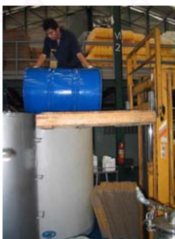
Figure 3.23 Inappropriate work method
