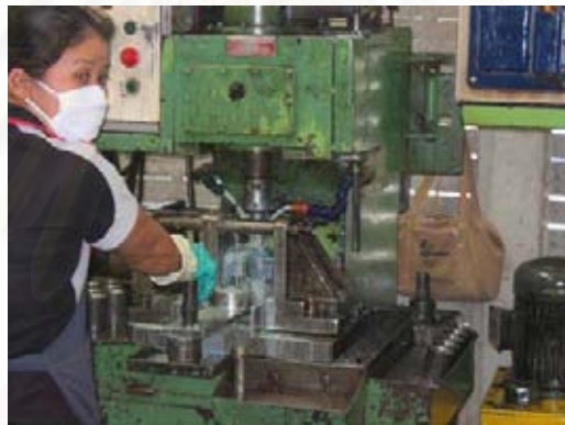
Figure 3.1 Application of metalworking lubricant (water soluble type)
