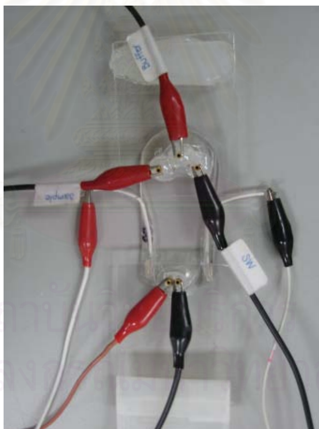
Figure 3.2 The microchip capillary electrophoresis with electrochemical detection layout.
