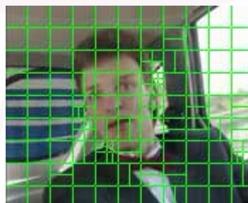
Figure 2.15 Frame divided into multiple macroblock of 16x16, 8x8, 8x4, 4x8 and 4x4 variable sizes to present different coding profiles.
