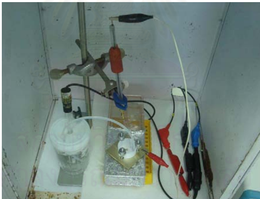
Figure 3.2 Electrochemical cell with BDD working electrode
