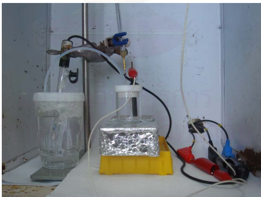
Figure 3.1 Electrochemical cell with Pt working electrode
