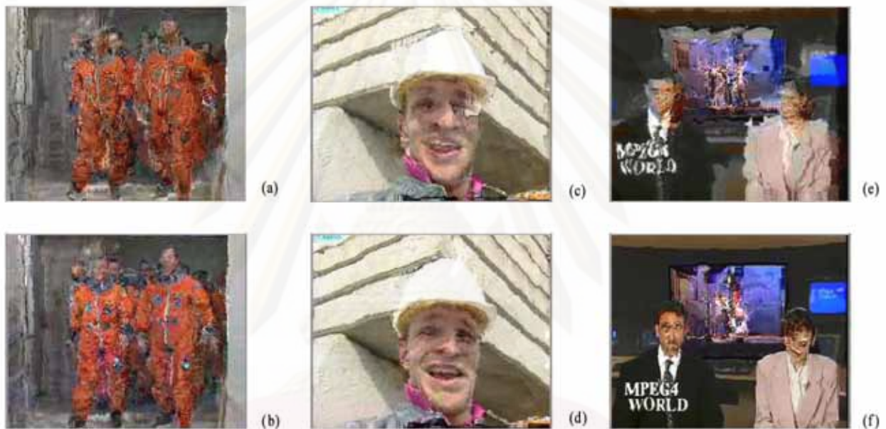
Figure 5. Subjective evaluation of the proposed algorithm and Frame Copy method. The frames above (a, c and e) were concealed using the frame copy method. The frames below ((b, d and f) were concealed using the proposed algorithm.
