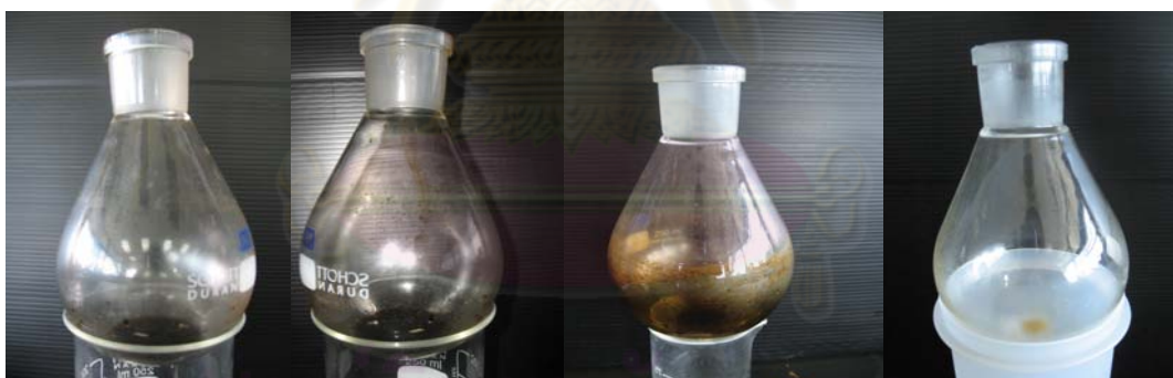
Figure 4.10 Characteristics of absolutes from four solvents: methanol, ethanol, ethyl acetate, and hexane in soxhlet extraction, respectively.
