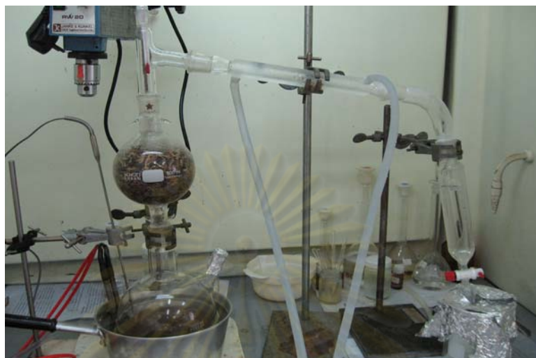
Figure 3.5 Steam distillation apparatus.
