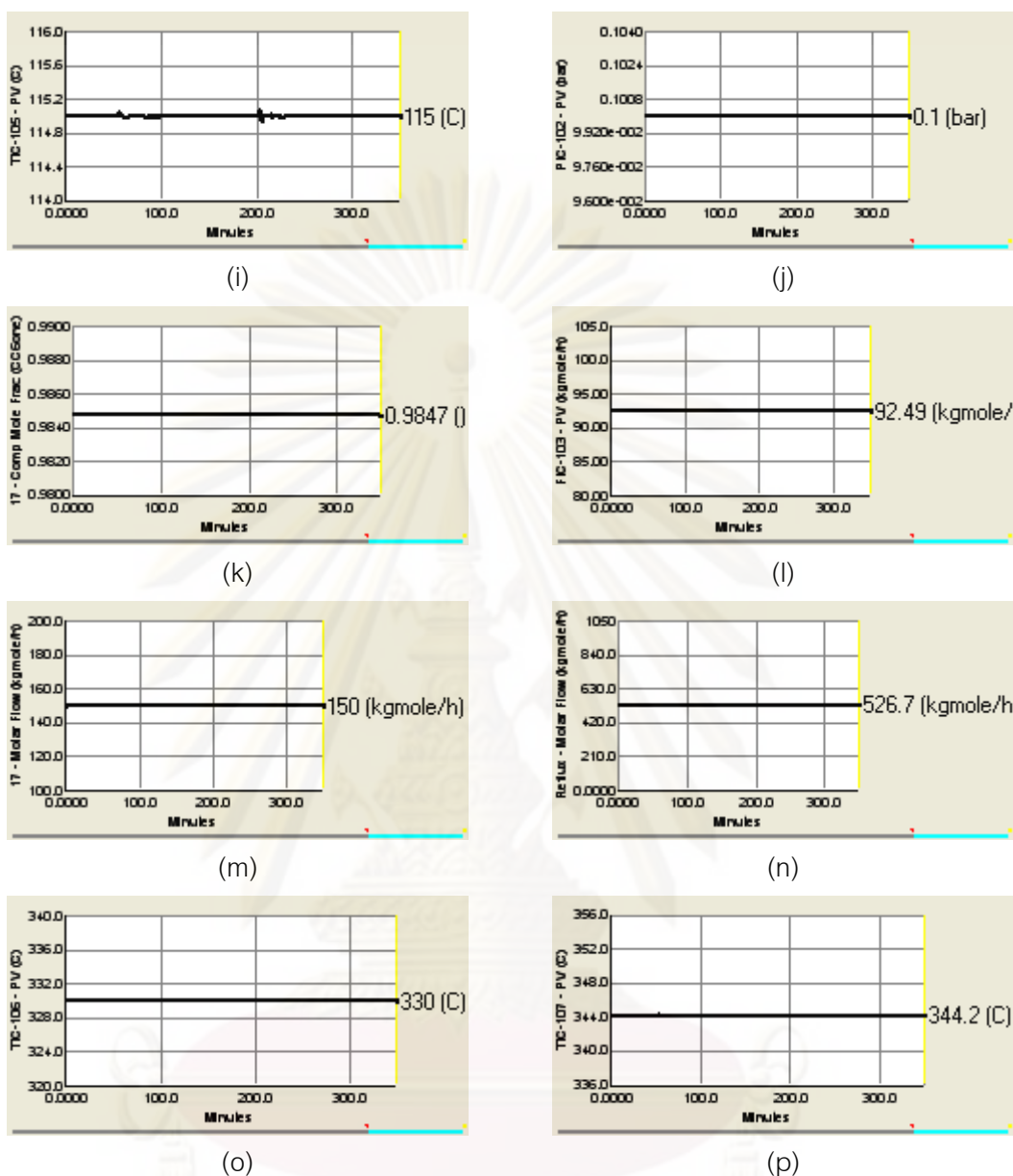
Figure 5.16 (Cont.) (i) cyclohexanone column feed temperature, (j) cyclohexanone column – condenser pressure, (k) cyclohexanol product composition, (l) cyclohexanone column – bottom flow, (m) cyclohexanone production flowrate, (n) cyclohexanone column – reflux flow (o) dehydrogenation reactor inlet temperature, (p) dehydrogenation reactor outlet temperature
