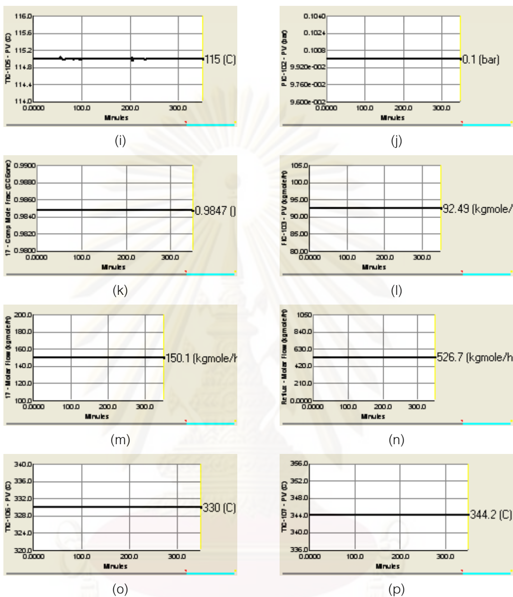
Figure 5.13 (Cont.) (i) cyclohexanone column feed temperature, (j) cyclohexanone column – condenser pressure, (k) cyclohexanol product composition, (l) cyclohexanone column – bottom flow, (m) cyclohexanone production flowrate, (n) cyclohexanone column – reflux flow (o) dehydrogenation reactor inlet temperature, (p) dehydrogenation reactor outlet temperature
