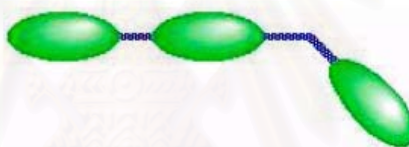
Figure 3.18 120- degree kinks in the polymer chain. [54]
