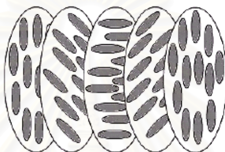
Figure 3.24 The structure of cholesteric phase. [53]
