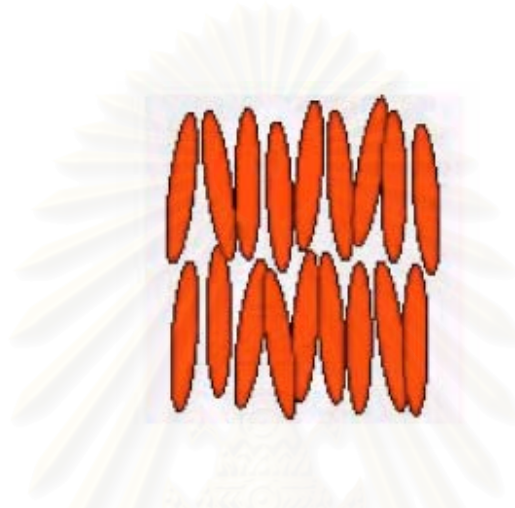
Figure 3.22 The structure of smectic phase. [53]
