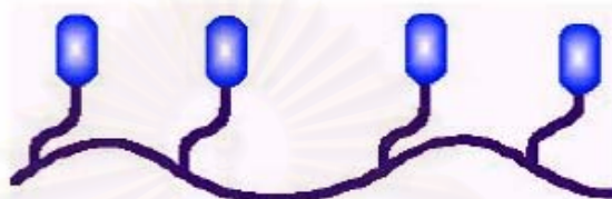
Figure 3.21 The tangle conformation and orientation of the mesogens. [54]
