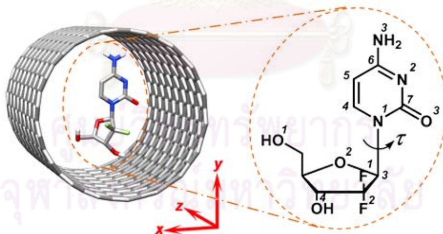
Figure 4.2 The structure of the (18,0) single-walled carbon nanotube (SWCNT) complexed with the gemcitabine drug where atomic labels and torsion angle ( \tau ) were also defined. The origin of the Cartesian coordinate for the complex was centered at the center of gravity ( C_g ) of the SWCNT.
