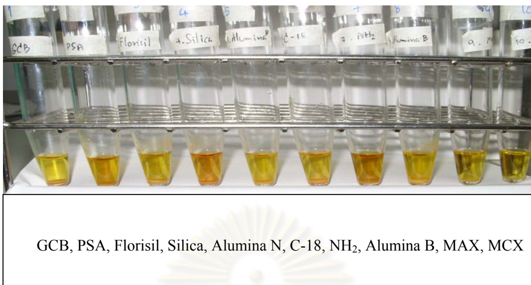
Figure 4.10 The extract samples after cleaned up and frozen at -20^{\circ}\text{C} overnight
