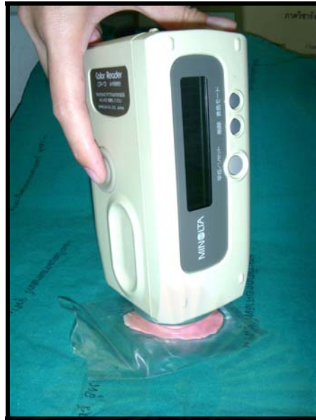
Figure12. Measuring the color of chewed gum by using the color reader
