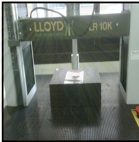
Figure10. Flattening chewed gum by compressing 10N-force
