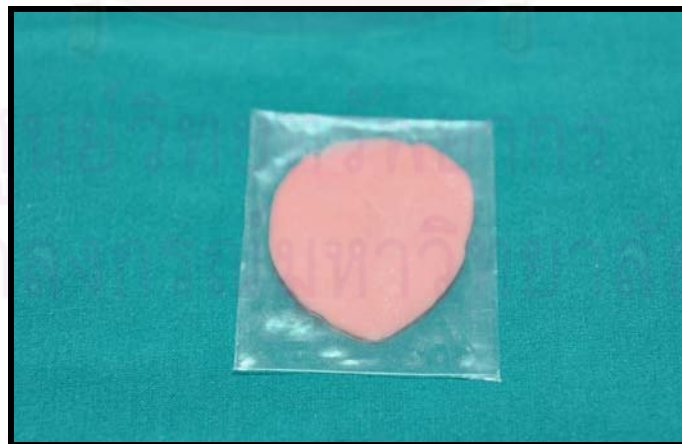
Figure11. The chewed gum after 1 mm. thickness flattening
