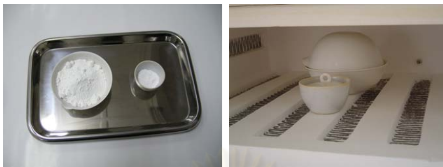
Figure 4.1: Preparation of raw materials for fabrication of ZnO target.
