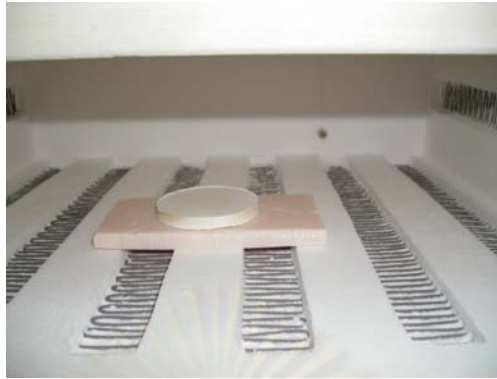
Figure 4.7: Sintering a target in a furnace.
