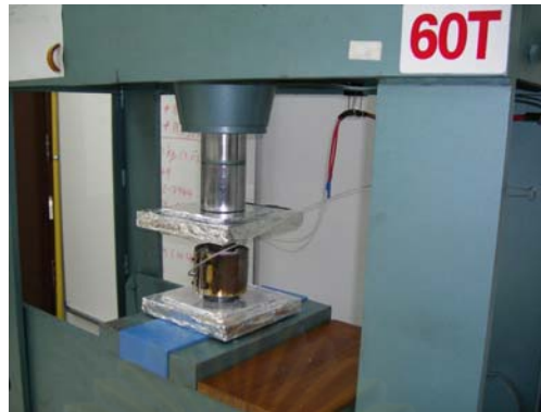
Figure 4.4: Pressing a target by hydrolic press with warming.
