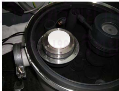
Figure 4.9: Installation of ZnO target in sputtering system.
