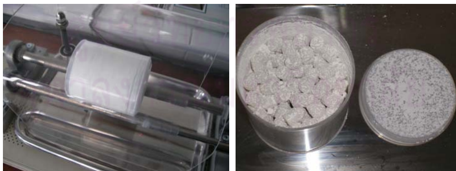
Figure 4.3: Ball milling of the raw material in a plastic container.
