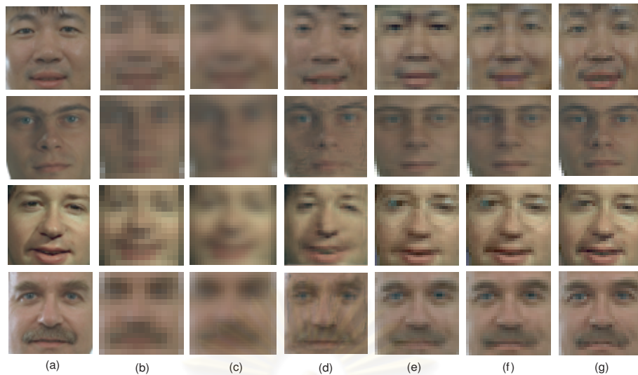
Figure 4.12: Color hallucinated face images, compared with other traditional methods in RGB color model. (a) original HR images ( 30 \times 30 ); (b) input LR images ( 15 \times 15 ) with noise, motion and blur in LR images; (c) face hallucination result with bilinear interpolation method; (d) face hallucination result with Liu method; (e) face hallucination result with 90 percent MPCA; (f) face hallucination result with 95 percent MPCA; (g) face hallucination result with 100 percent MPCA;
