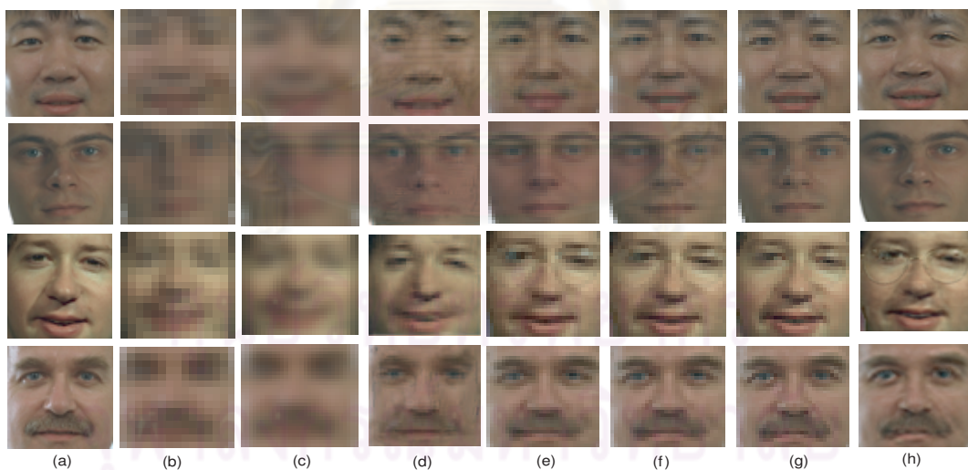
Figure 4.50: Color hallucinated face images in CIELAB color model. (a) original HR images ( 30 \times 30 ); (b) input LR images ( 15 \times 15 ) with noise, motion and blur in LR images; (c) face hallucination result with bilinear interpolation method; (d) face hallucination result with Liu method; (e) face hallucination result with 90 percent MPCA; (f) face hallucination result with 95 percent MPCA; (g) face hallucination result with 100 percent MPCA; (h) face hallucination result with Tensor ( 5 \times 5 ) patches method and 95 percent MPCA;
