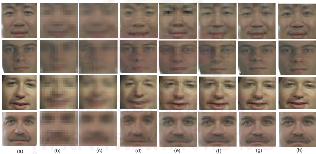
Figure 4.56: Color hallucinated face images in YCbCr color model. (a) original HR images ( 30 \times 30 ); (b) input LR images ( 15 \times 15 ) with noise, motion and blur in LR images; (c) face hallucination result with bilinear interpolation method; (d) face hallucination result with Liu method; (e) face hallucination result with 90 percent MPCA; (f) face hallucination result with 95 percent MPCA; (g) face hallucination result with 100 percent MPCA; (h) face hallucination result with Tensor ( 10 \times 10 ) patches method and 100 percent MPCA;
