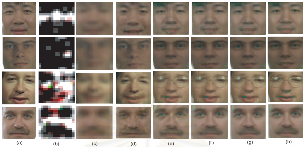
Figure 4.57: Color hallucinated face images in HSV color model. (a) original HR images ( 30 \times 30 ); (b) input LR images ( 15 \times 15 ) with noise, motion and blur in LR images; (c) face hallucination result with bilinear interpolation method; (d) face hallucination result with Liu method; (e) face hallucination result with 90 percent MPCA; (f) face hallucination result with 95 percent MPCA; (g) face hallucination result with 100 percent MPCA; (h) face hallucination result with Tensor ( 10 \times 10 ) patches method and 100 percent MPCA;
