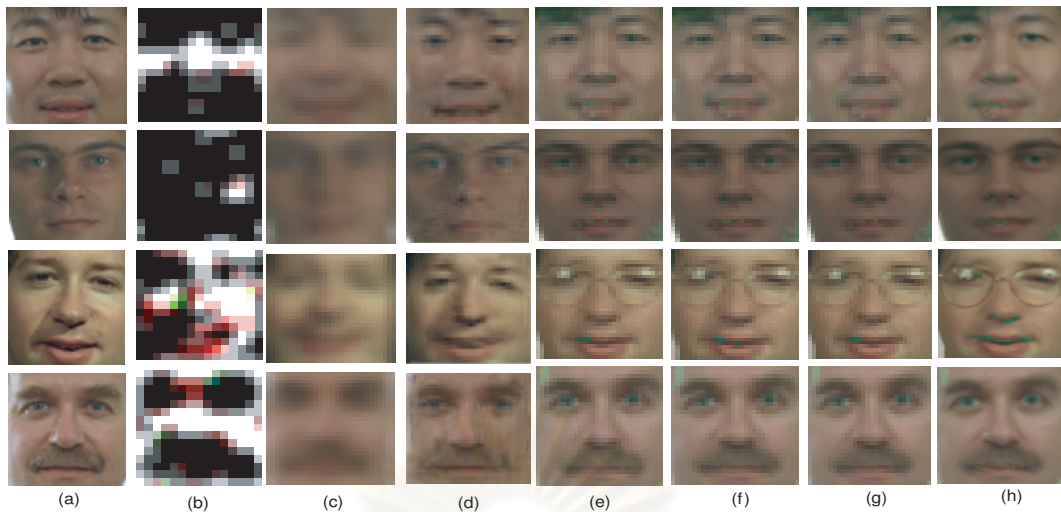
Figure 4.45: Color hallucinated face images in HSV color model. (a) original HR images ( 30 \times 30 ); (b) input LR images ( 15 \times 15 ) with noise, motion and blur in LR images; (c) face hallucination result with bilinear interpolation method; (d) face hallucination result with Liu method; (e) face hallucination result with 90 percent MPCA; (f) face hallucination result with 95 percent MPCA; (g) face hallucination result with 100 percent MPCA; (h) face hallucination result with Tensor ( 5 \times 5 ) patches method and 95 percent MPCA;
