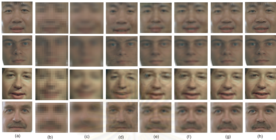
Figure 4.58: Color hallucinated face images in CIELAB color model. (a) original HR images ( 30 \times 30 ); (b) input LR images ( 15 \times 15 ) with noise, motion and blur in LR images; (c) face hallucination result with bilinear interpolation method; (d) face hallucination result with Liu method; (e) face hallucination result with 90 percent MPCA; (f) face hallucination result with 95 percent MPCA; (g) face hallucination result with 100 percent MPCA; (h) face hallucination result with Tensor ( 10 \times 10 ) patches method and 100 percent MPCA;
