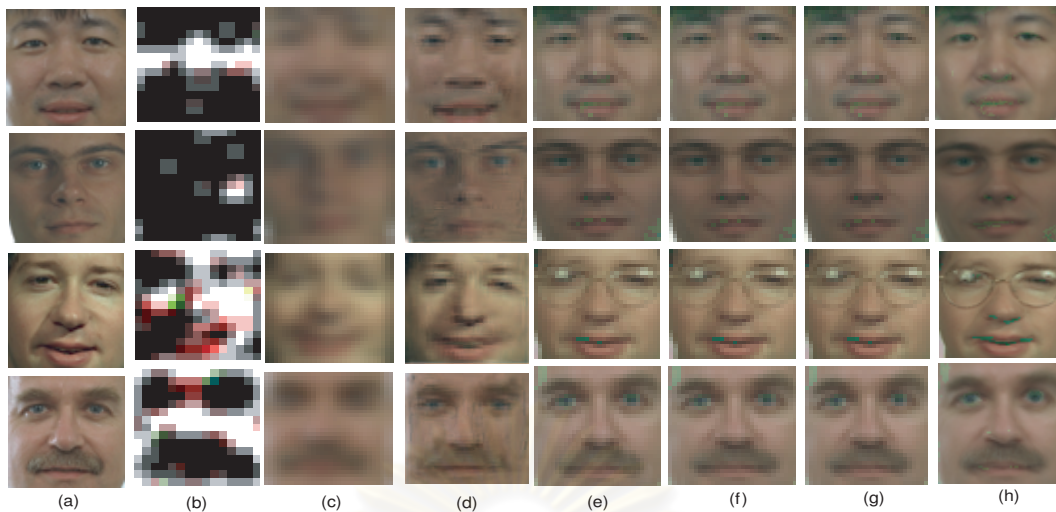
Figure 4.53: Color hallucinated face images in HSV color model. (a) original HR images ( 30 \times 30 ); (b) input LR images ( 15 \times 15 ) with noise, motion and blur in LR images; (c) face hallucination result with bilinear interpolation method; (d) face hallucination result with Liu method; (e) face hallucination result with 90 percent MPCA; (f) face hallucination result with 95 percent MPCA; (g) face hallucination result with 100 percent MPCA; (h) face hallucination result with Tensor ( 10 \times 10 ) patches method and 95 percent MPCA;
