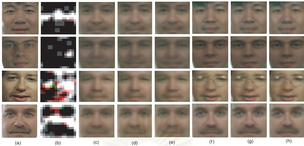
Figure 4.10: Color hallucinated face images in HSV color model. (a) original HR images ( 30 \times 30 ); (b) input LR images ( 15 \times 15 ) with noise, motion and blur in LR images; (c) face hallucination result with 90 percent traditional PCA; (d) face hallucination result with 95 percent traditional PCA; (e) face hallucination result with 100 percent traditional PCA; (f) face hallucination result with 90 percent MPCA; (g) face hallucination result with 95 percent MPCA; (h) face hallucination result with 100 percent MPCA;
