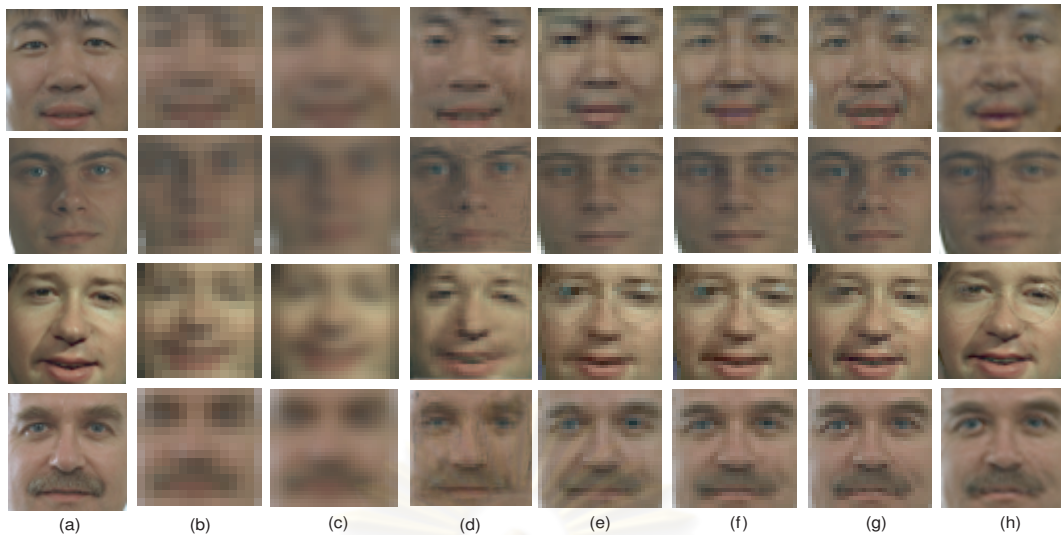
Figure 4.51: Color hallucinated face images in RGB color model. (a) original HR images ( 30 \times 30 ); (b) input LR images ( 15 \times 15 ) with noise, motion and blur in LR images; (c) face hallucination result with bilinear interpolation method; (d) face hallucination result with Liu method; (e) face hallucination result with 90 percent MPCA; (f) face hallucination result with 95 percent MPCA; (g) face hallucination result with 100 percent MPCA; (h) face hallucination result with Tensor ( 10 \times 10 ) patches method and 95 percent MPCA;
