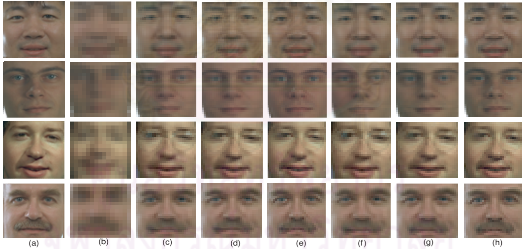
Figure 4.19: Color hallucinated face images, compared between TensorPCA and MPCA in CIELAB color model. (a) original HR images ( 30 \times 30 ); (b) input LR images ( 15 \times 15 ) with noise, motion and blur in LR images; (c) face hallucination result with 90 percent tensorPCA; (d) face hallucination result with 95 percent tensorPCA; (e) face hallucination result with 100 percent tensorPCA; (f) face hallucination result with 90 percent MPCA; (g) face hallucination result with 95 percent MPCA; (h) face hallucination result with 100 percent MPCA;
