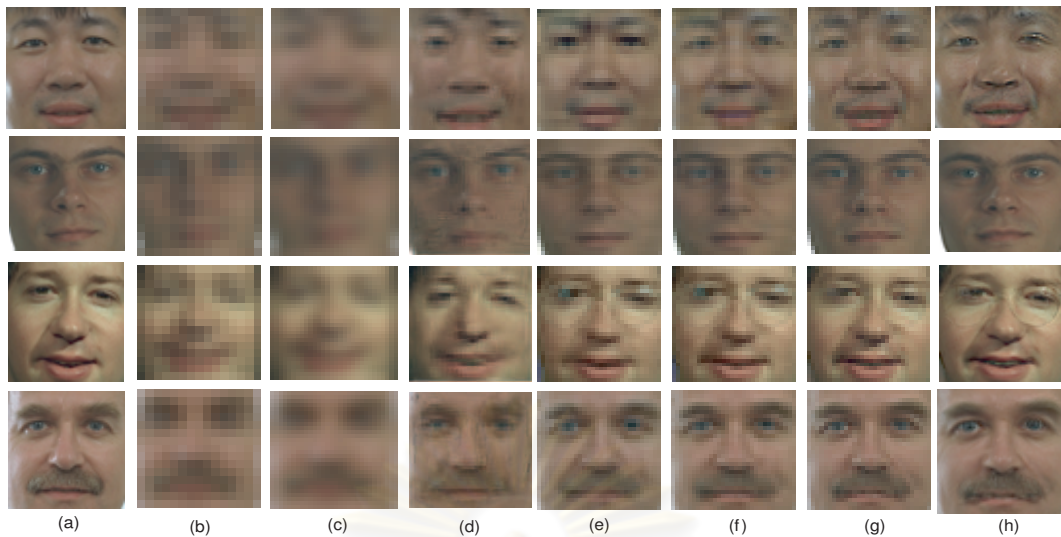
Figure 4.47: Color hallucinated face images in RGB color model. (a) original HR images ( 30 \times 30 ); (b) input LR images ( 15 \times 15 ) with noise, motion and blur in LR images; (c) face hallucination result with bilinear interpolation method; (d) face hallucination result with Liu method; (e) face hallucination result with 90 percent MPCA; (f) face hallucination result with 95 percent MPCA; (g) face hallucination result with 100 percent MPCA; (h) face hallucination result with Tensor ( 5 \times 5 ) patches method and 100 percent MPCA;
