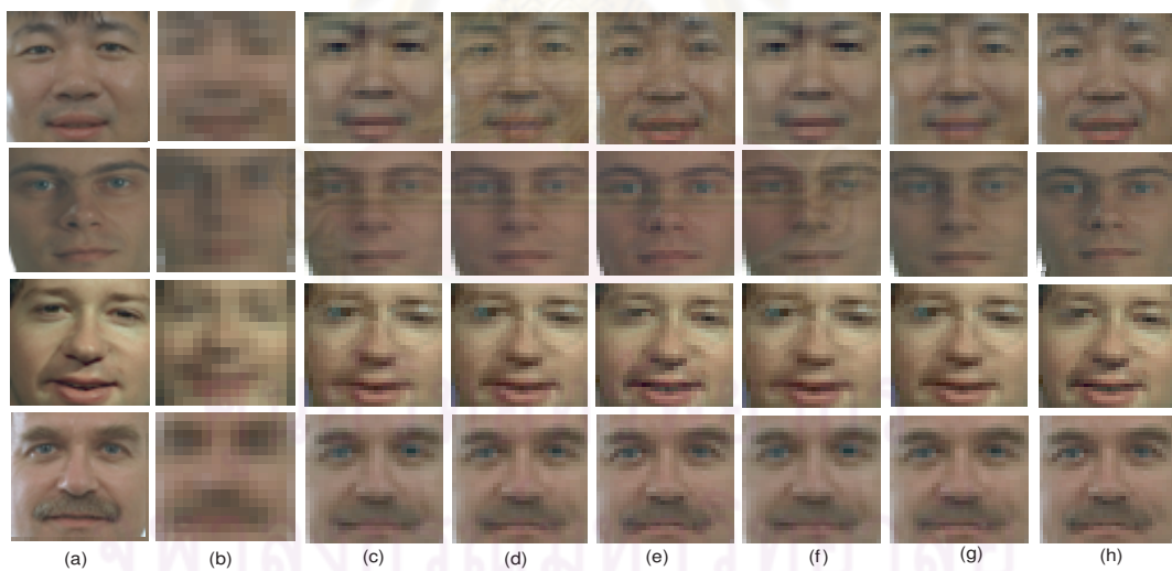
Figure 4.17: Color hallucinated face images, compared between TensorPCA and MPCA in YCbCr color model. (a) original HR images ( 30 \times 30 ); (b) input LR images ( 15 \times 15 ) with noise, motion and blur in LR images; (c) face hallucination result with 90 percent tensorPCA; (d) face hallucination result with 95 percent tensorPCA; (e) face hallucination result with 100 percent tensorPCA; (f) face hallucination result with 90 percent MPCA; (g) face hallucination result with 95 percent MPCA; (h) face hallucination result with 100 percent MPCA;
