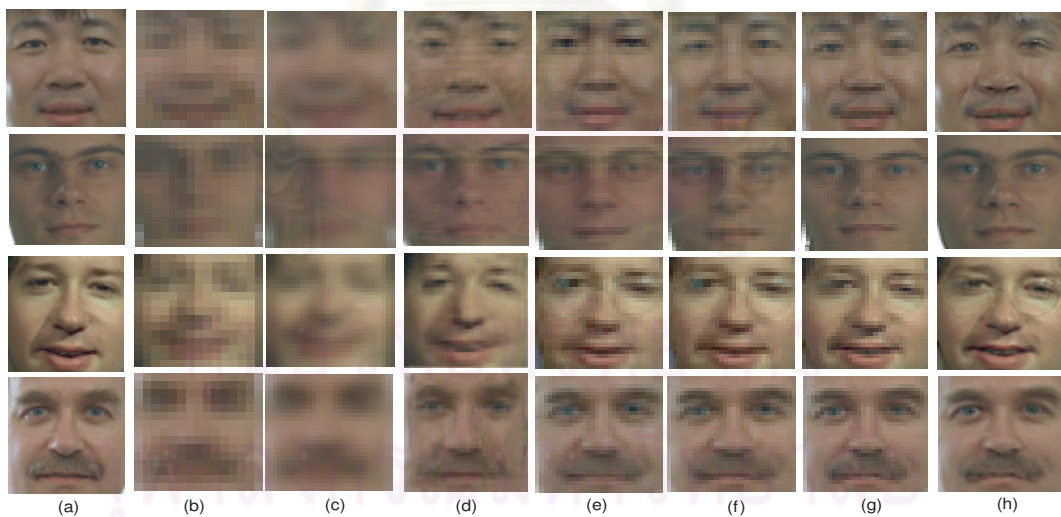
Figure 4.48: Color hallucinated face images in YCbCr color model. (a) original HR images ( 30 \times 30 ); (b) input LR images ( 15 \times 15 ) with noise, motion and blur in LR images; (c) face hallucination result with bilinear interpolation method; (d) face hallucination result with Liu method; (e) face hallucination result with 90 percent MPCA; (f) face hallucination result with 95 percent MPCA; (g) face hallucination result with 100 percent MPCA; (h) face hallucination result with Tensor ( 5 \times 5 ) patches method and 100 percent MPCA;
