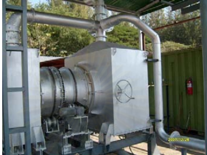
Figure A-1 Pilot-scale rotary cement kiln
