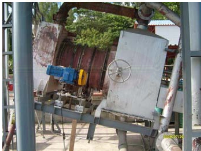
Figure A- 2 Pilot scale-rotary cement kiln was rose up to remove some residue
