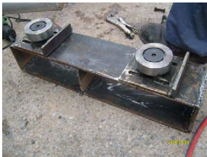
Figure A-11 Roller for moving the rotary kiln
