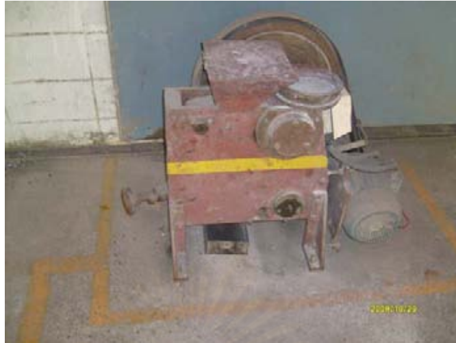
Figure B-6 Grinding machine for reducing size of clinker sample
