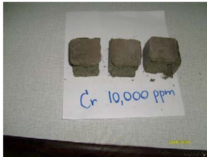
Figure C-15 Cement mortar contained 10,000 ppm of Cr
