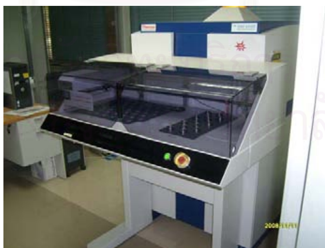
Figure B-5 Combination machine of XRF and XRD
