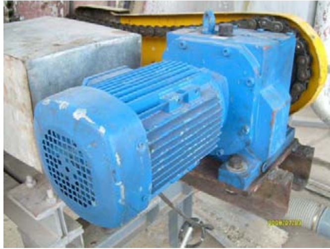
Figure A-12 The 1 horse power of motor for driving the rotary kiln
