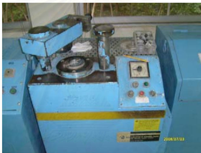
Figure B-4 Tablet machine for using in the combination machine of XRF and XRD
