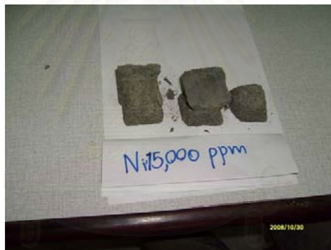
Figure C-31 Cement mortar contained 15,000 ppm of Ni
