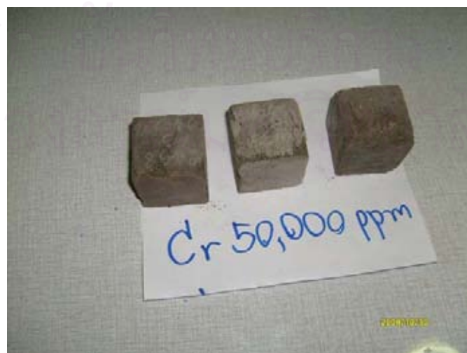
Figure C-17 Cement mortar contained 50,000 ppm of Cr
