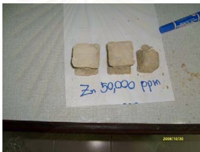
Figure C-42 Cement mortar contained 50,000 ppm of Zn
