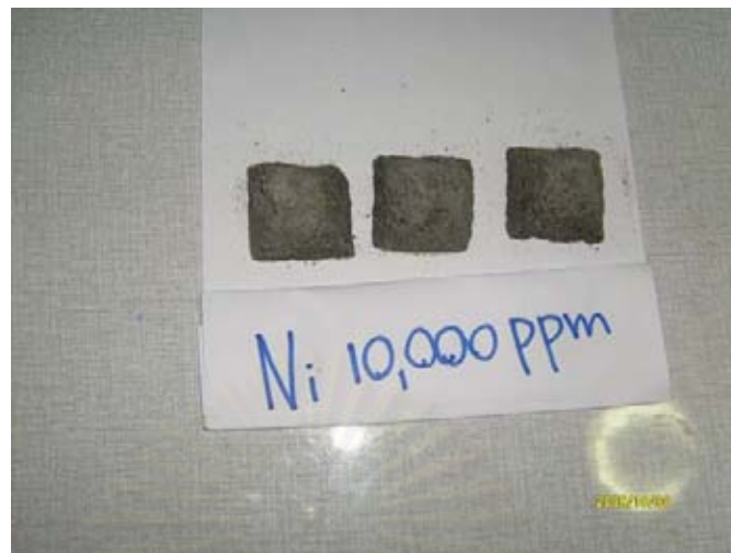
Figure C-30 Cement mortar contained 10,000 ppm of Ni
