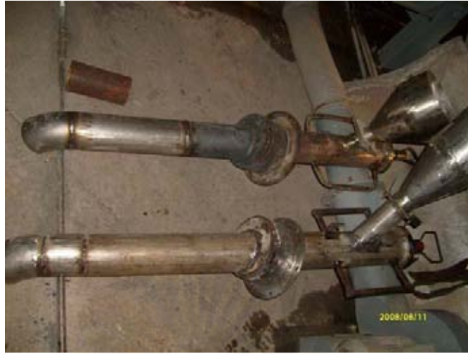
Figure A-9 Stainless steel type 235 capsules for adding sample
