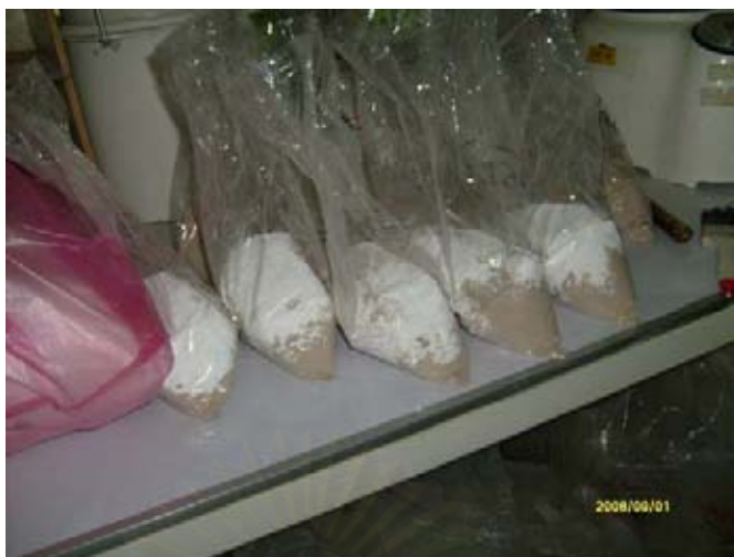
Figure C-38 The mixtures of kiln feeds and zinc oxide before mixing by V-mix machine
