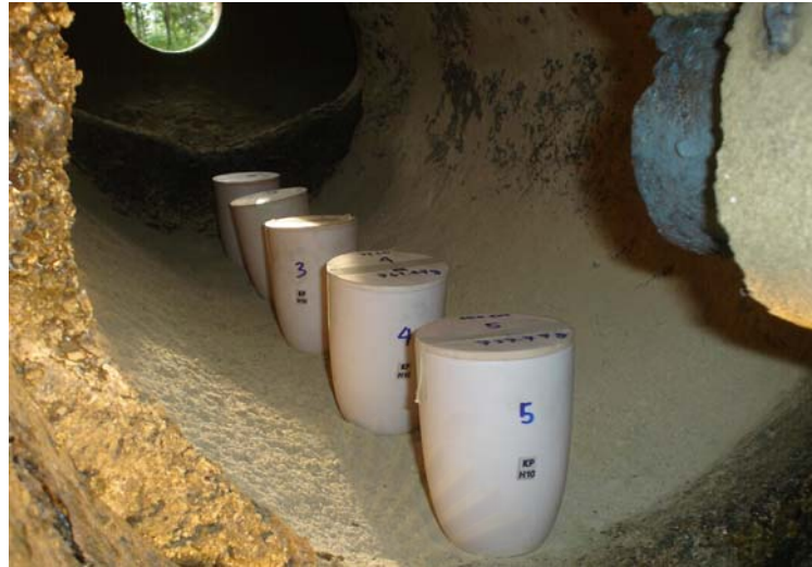
Figure 4.4: The positioning of the five crucible glasses for the static burning process
