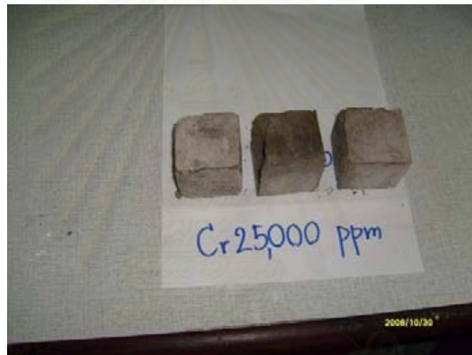
Figure C-16 Cement mortar contained 25,000 ppm of Cr
