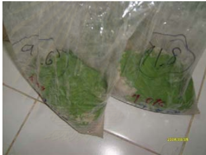
Figure C-13 Mixture of kiln feed and chromium (III) oxide before mixing by V-mix machine
