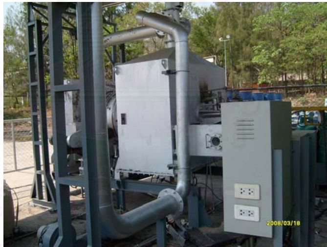
Figure 3.1: Pilot- scale rotary cement kiln
