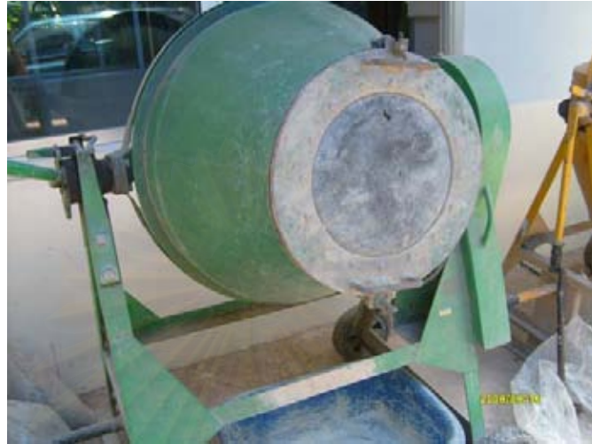
Figure B-1 Mixing machine for mixing between each collected raw meal
