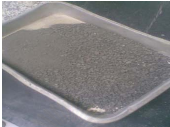
Figure C-5 Clinker after crushed by the grinding machine
