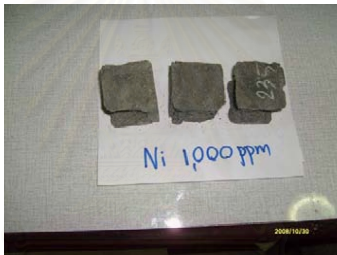
Figure C-28 Cement mortar contained 1,000 ppm of Ni
