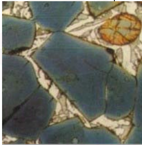
Figure 2.5: Photomicrograph of clinker (0.11mm.) that contain alite (blue), belite (orange), tricalcium aluminium (grey), and ferrite (white).
