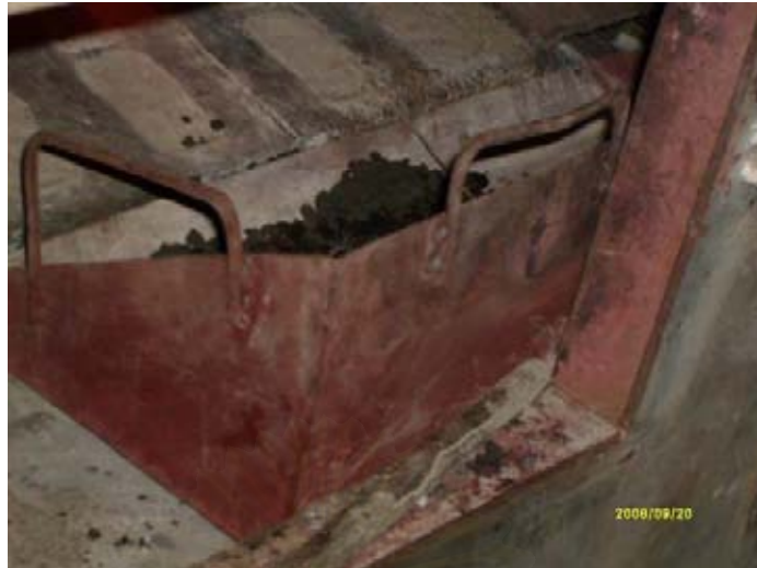
Figure 4.5: Clinker inside the pilot-scale rotary cement kiln
