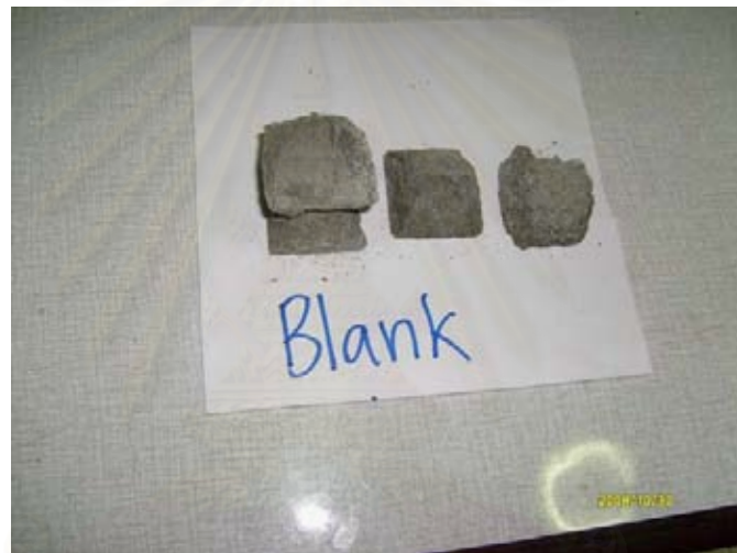
Figure C-6 Cement mortar control after compressed by the compressive machine
