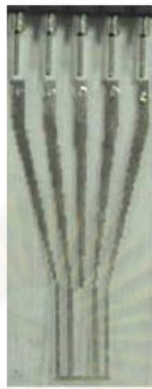
Figure 2. 15 Sensor material coated onto a plastic (Parikh et al. 2006).
