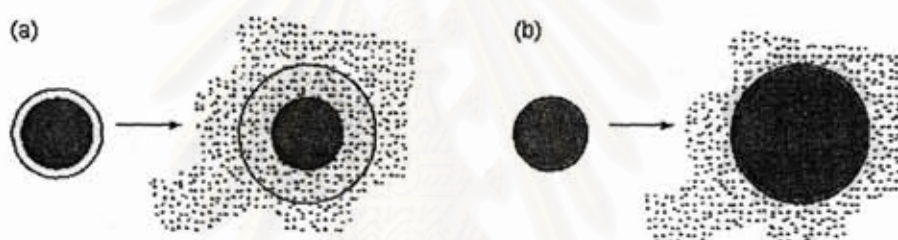
Figure 2.7 Drug delivery from (a) reservoir and (b) matrix swelling-controlled release systems.
