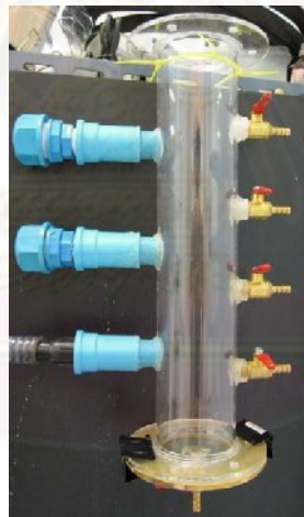
Figure 3.3 Decantation column employed in this study
