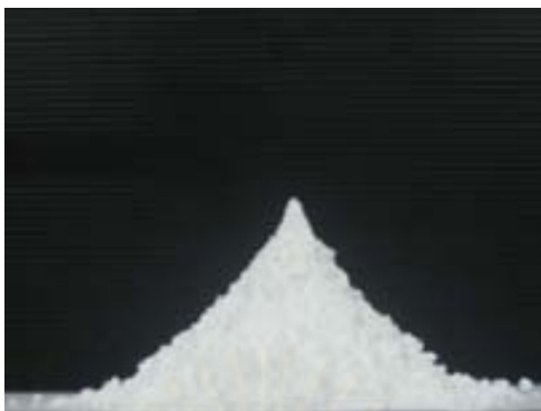
Figure C4 Spray dried products for condition, inlet temperature 120°C, feed rate 3.5 ml/min): Angle of repose = 40°
