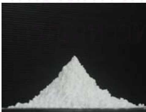
Figure C6 Spray dried products for condition, inlet temperature 120°C, feed rate 10.5 ml/min): Angle of repose = 45°
