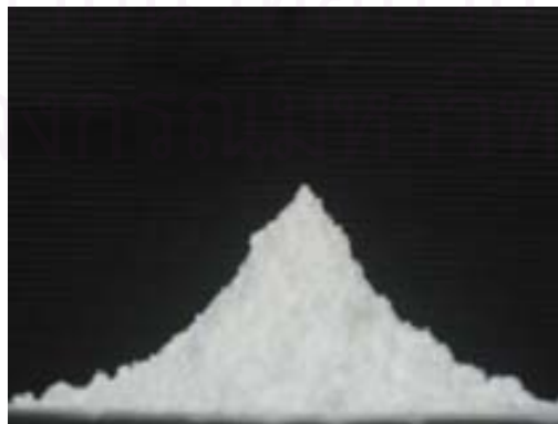
Figure C3 Spray dried products for condition, inlet temperature 100°C, feed rate 10.5 ml/min): Angle of repose = 40°
