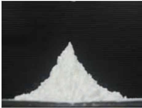
Figure C1 Spray dried products for condition, inlet temperature 100°C, feed rate 3.5 ml/min) :Angle of repose = 50°
