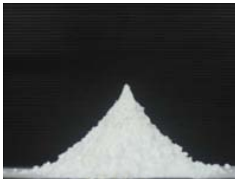
Figure C7 Spray dried products for condition, inlet temperature 140°C, feed rate 3.5 ml/min): Angle of repose = 45°
