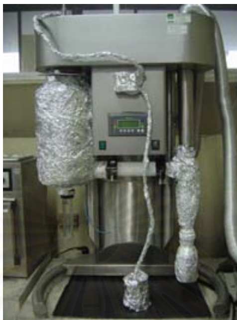
Figure7. Light protection during the drying process
