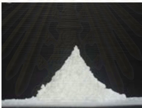
Figure C5 Spray dried products for condition, inlet temperature 120°C, feed rate 7.0 ml/min): Angle of repose = 50°
