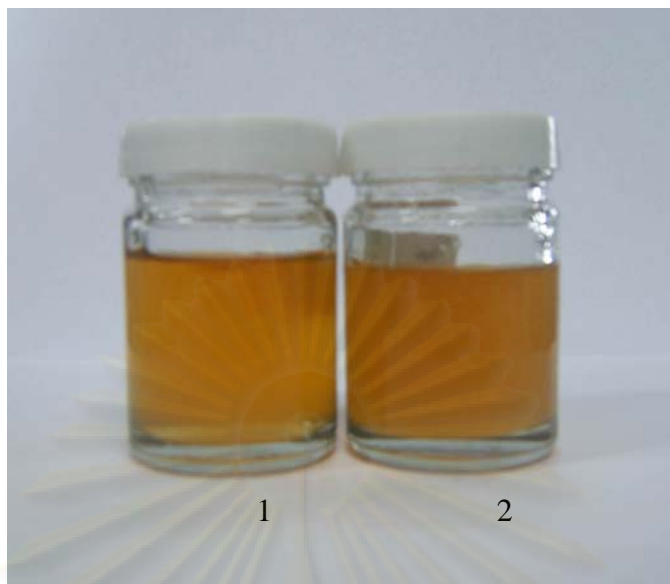
Figure 18. PG gel with TSCE 140 \mu\text{g/g} (Formulation 3): 1 = After 30 days at ambient temperature 2 = After 4 cycles of temperature cycling test
