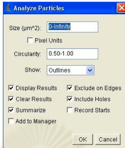
Figure 3.8 Parameter settings in analysis of proton tracks as seen on the screen of the ImageJ software.
