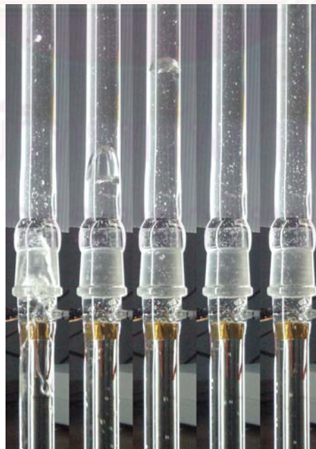
Fig. 5.14 Recorded bubble images at the heater outlet
