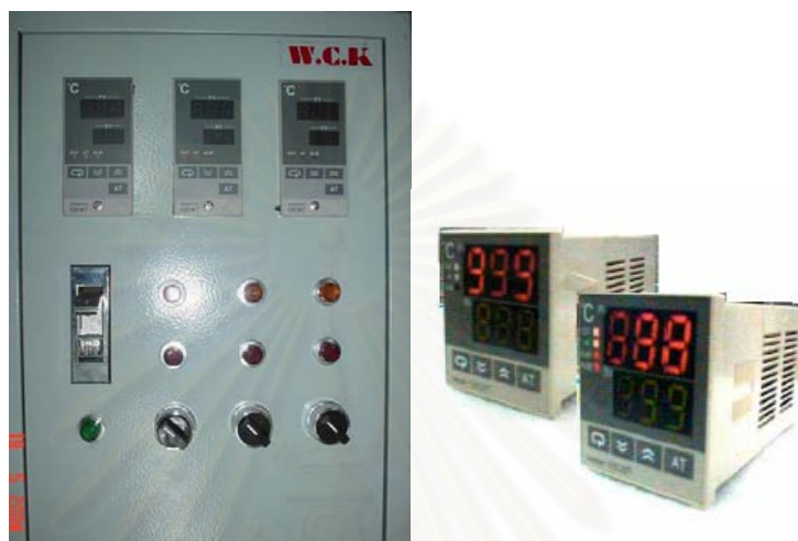
Figure 4.6 The temperature control system
