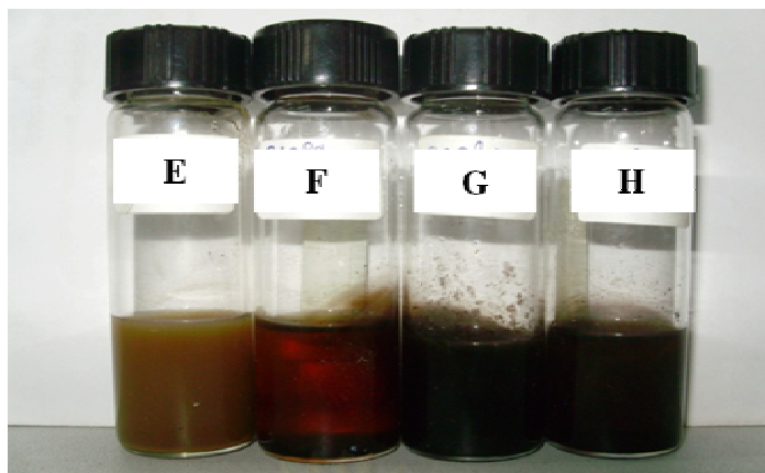
Figure 5.7.2 Liquid samples after hydrothermal treatment with the concentration of feedstock at 20 wt % and 7.5 °C/min. (E) 220 °C, (F) 260 °C, (G) 280 °C and (H) 300 °C
