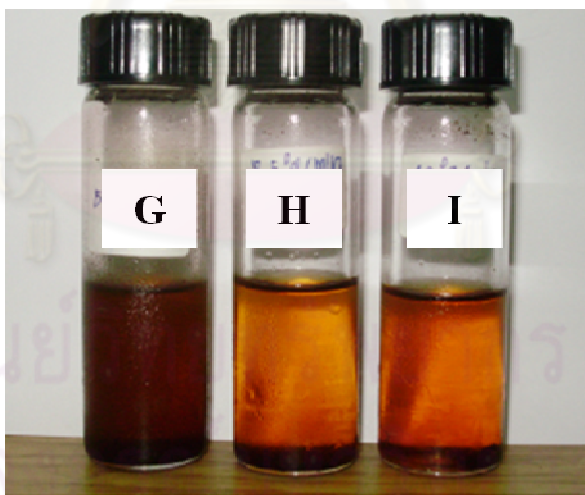
Figure 5.6.3 Liquid samples after hydrothermal treatment at 280 °C with heating rate of (G) 5 °C/min, (H) 7.5 °C/min and (I) 10 °C/min
