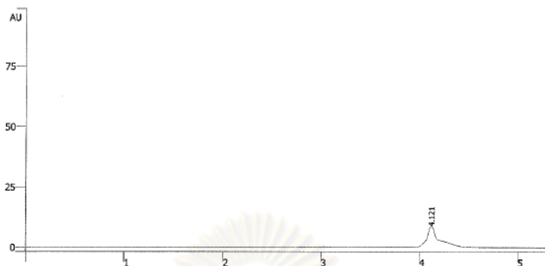
Figure A21 HPLC chromatogram of 5-HMF solution at 2,600 ppm, 5 \mu l, area 761,128,448 counts
