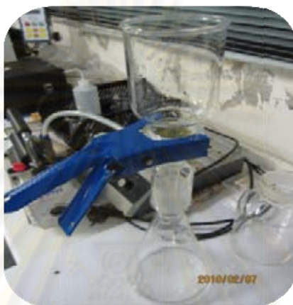
Figure 4.3.3 Liquid-solid filtration systems
