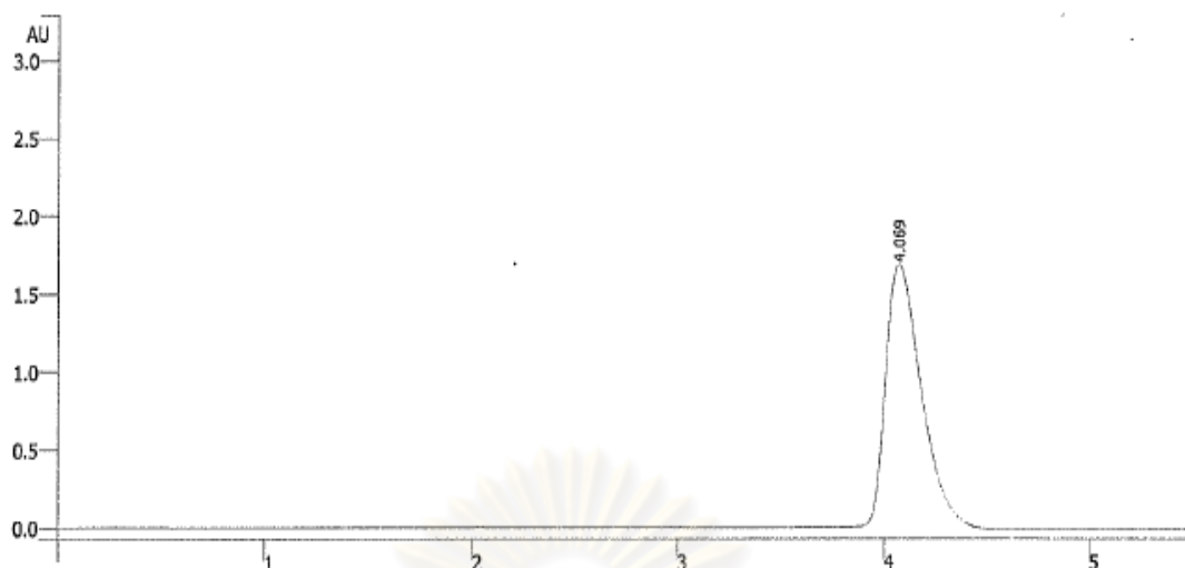
Figure A9 HPLC chromatogram of 5-HMF solution at 200 ppm, 5 \mu l, area 191,403,792 counts
