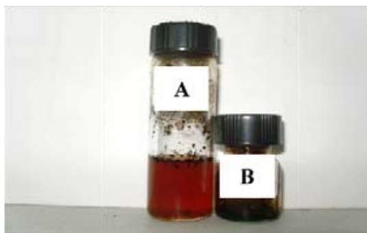
Figure 5.12.3 Liquid samples after hydrothermal treatment in the presence of 20 v/v% of DMSO and 2-butanol under 280 °C and 5 °C/min (A) aqueous phase and (B) extracting phase
