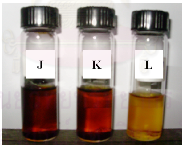
Figure 5.6.4 Liquid samples after hydrothermal treatment at 300 °C with heating rate of (J) 5 °C/min, (K) 7.5 °C/min and (L) 10 °C/min
