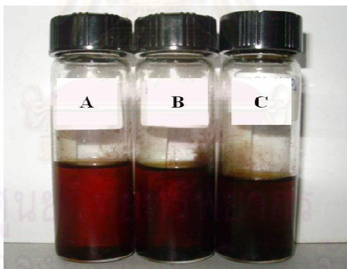
Figure 5.11.1 Liquid samples after hydrothermal treatment in the presence of \text{H}_3\text{PO}_4 under 280 °C and 5 °C/min (A) 1 v/v%, (B) 3 v/v% and (C) 5 v/v%
