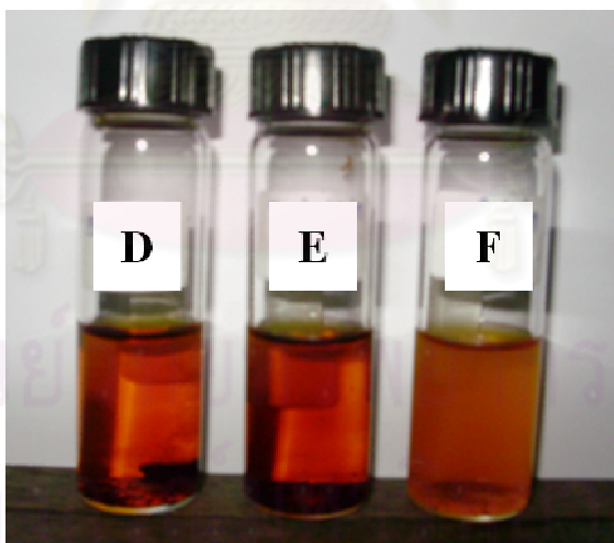
Figure 5.6.2 Liquid samples after hydrothermal treatment at 260 °C with heating rate of (D) 5 °C/min, (E) 7.5°C/min and (F) 10 °C/min
