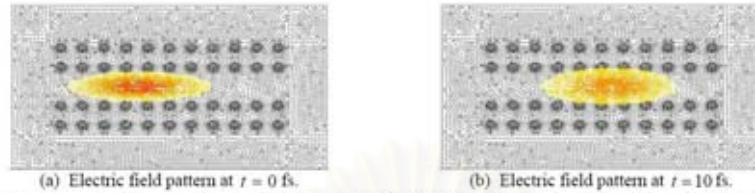
Figure 6 The initial pulse at t = 0 fs. (a) and the pulse propagation at t = 10 fs. with using polygonal elements mesh (b)
