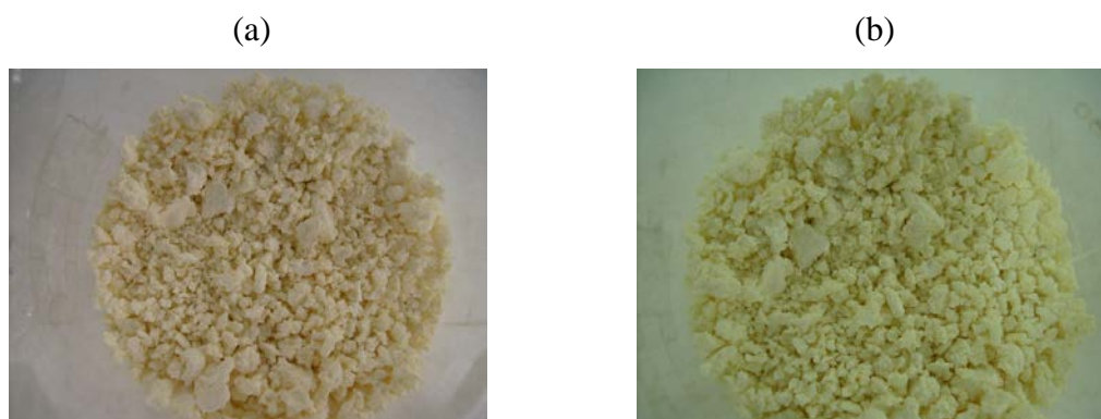
Figure A.4 Appearance of (a) Ce-ZnO (P) 1:2 and (b) Ce-ZnO (S) 1:2 after calcination.
