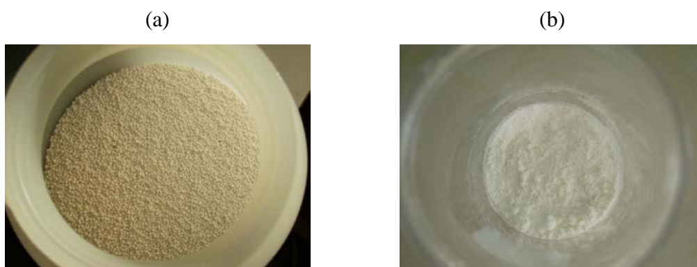
Figure A.1 Raw material images: (a) \text{Al}_2\text{O}_3 beads and (b) commercial ZnO powder.
