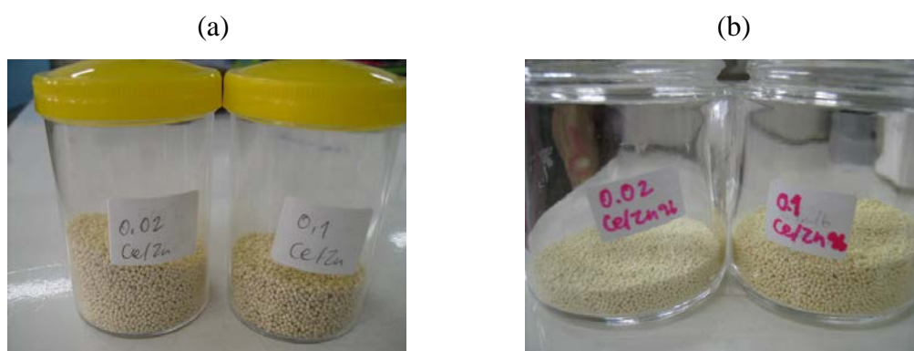
Figure A.5 Appearance of (a) Ce-ZnO (P) 1:2 and (b) Ce-ZnO (S) 1:2 beads.
