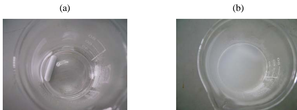
Figure A.3 Appearance of (a) 0.02Ce-ZnO polyvinylpyrrolidone gel and (b) 0.02Ce-ZnO starch gel.
