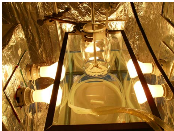
Figure D.2 Reactor for photocatalytic degradation of atrazine under visible light irradiation as described the procedure in 3.4.2 and the experimental result in 4.1.2.2.
