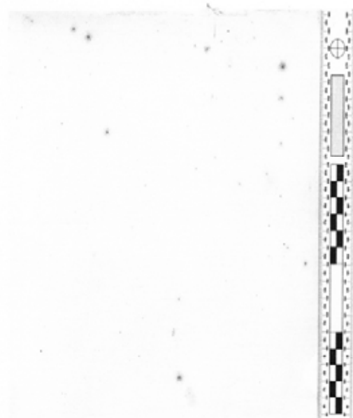
Fig. 8. Visualized gunpowder residue transferred to the wet polyester textile from the brown wrapping paper at the firing distance of 75–100 cm.
