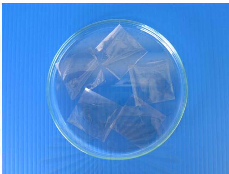
Figure 8. PG dressing films prepared from polysaccharide gel (PG) by a casting/solvent evaporating technique.
