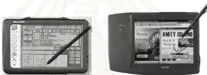
a) Hand held PDA (Sharp Zaurus [160]) b) Pen-based portable computer (Mitsubishi AMiTY [2])
