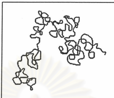
Figure 2.10 Random coil model of bulk amorphous polymer [Grassino, 2000]
