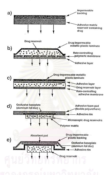
Figure 6 Cross-section views of transdermal delivery system
