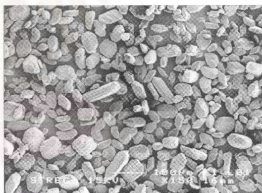
Mae Moh FGD gypsum (precleaned)
