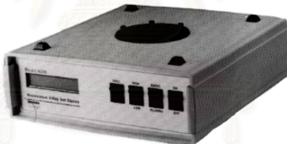
Figure 4: Digital ionization chamber (Victoreen model 4000M + )
