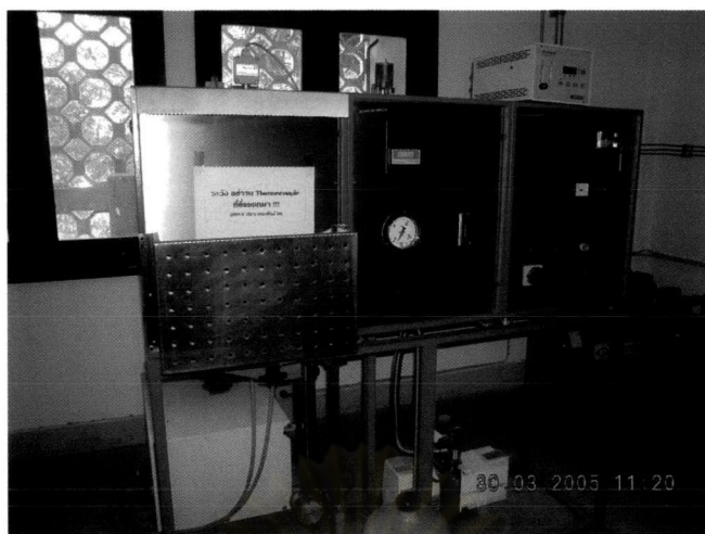
Figure 6.1 The furnace used in this experiment is Linn electrical furnace model HT 1800 Plus VAC Bottom Loader (Chulalongkorn University).
