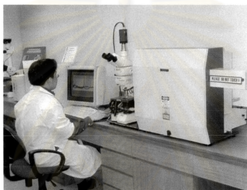
Figure 3.14 Laser Raman Spectroscope belonging to the GIT used for identification of mineral inclusion.
