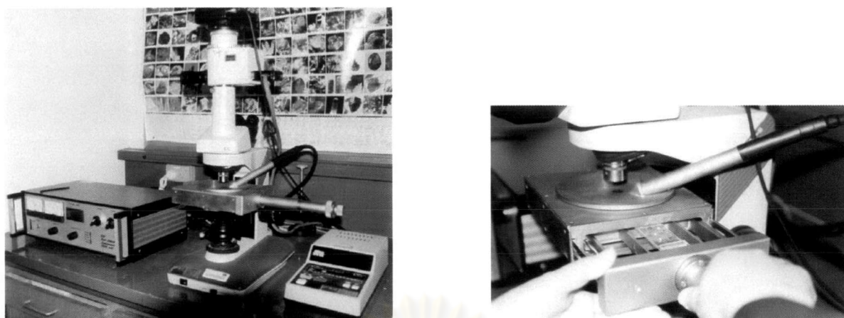
Figure 3.5 Cathodoluminescope; model CLmk3A, Cambridge Image Technology Limited, based at Kasetsart University.
