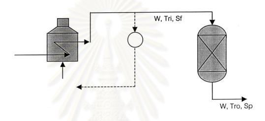
Figure 4.1 The hydro-desulphurisation process for this study
